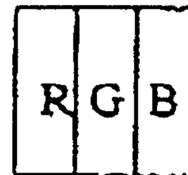
Typical 300um square pixel divided into 3 coloured sub-pixels
