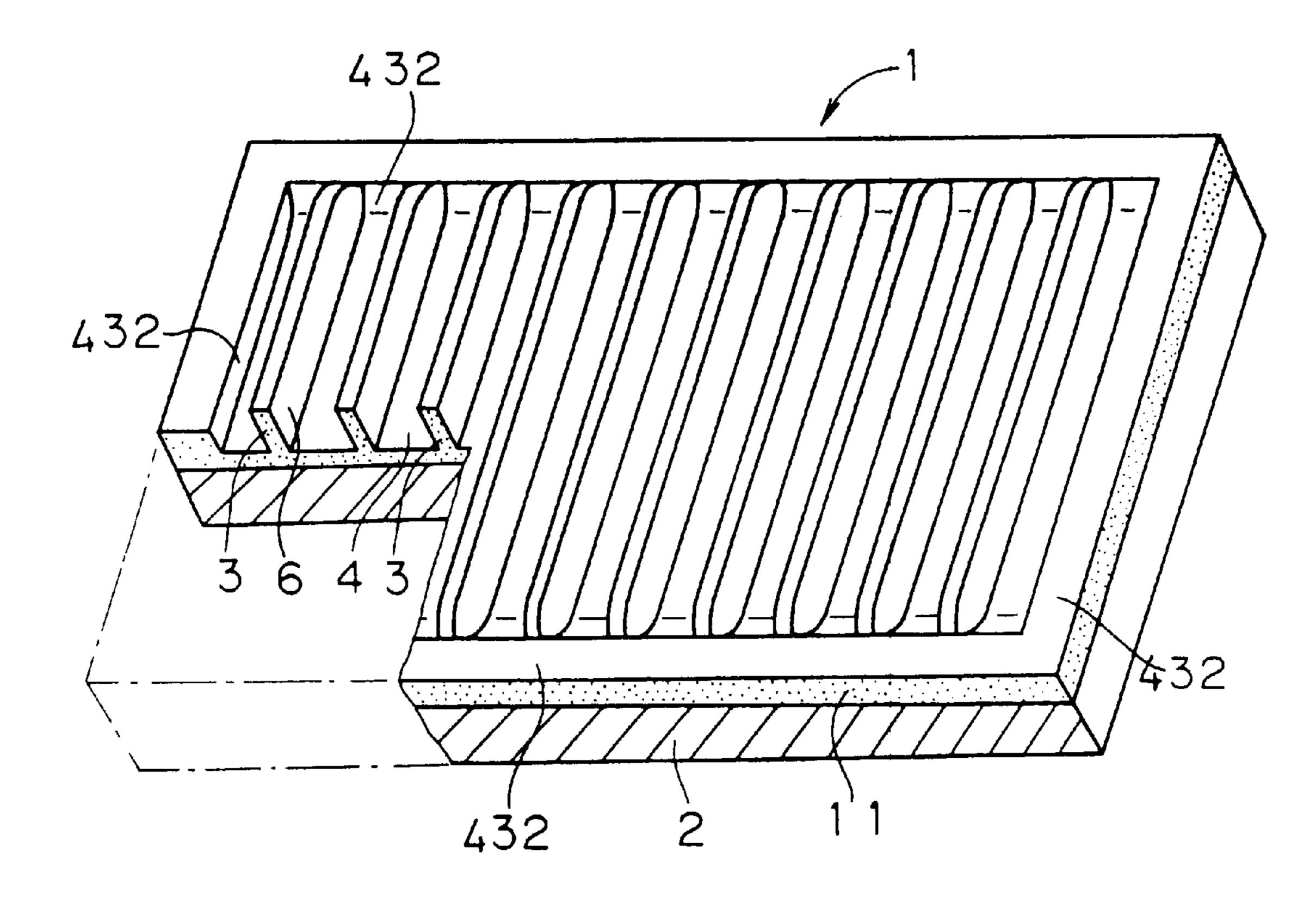
METHOD FOR MANUFACTURING FLAT PLATE WITH PRECISE BULKHEAD, FLAT PLATE WITH PRECISE BULKHEAD, METHOD FOR MANUFACTURING PLASMA DISPLAY UNIT SUBSTRATE AND PLASMA DISPLAY UNIT SUBSTRATE
