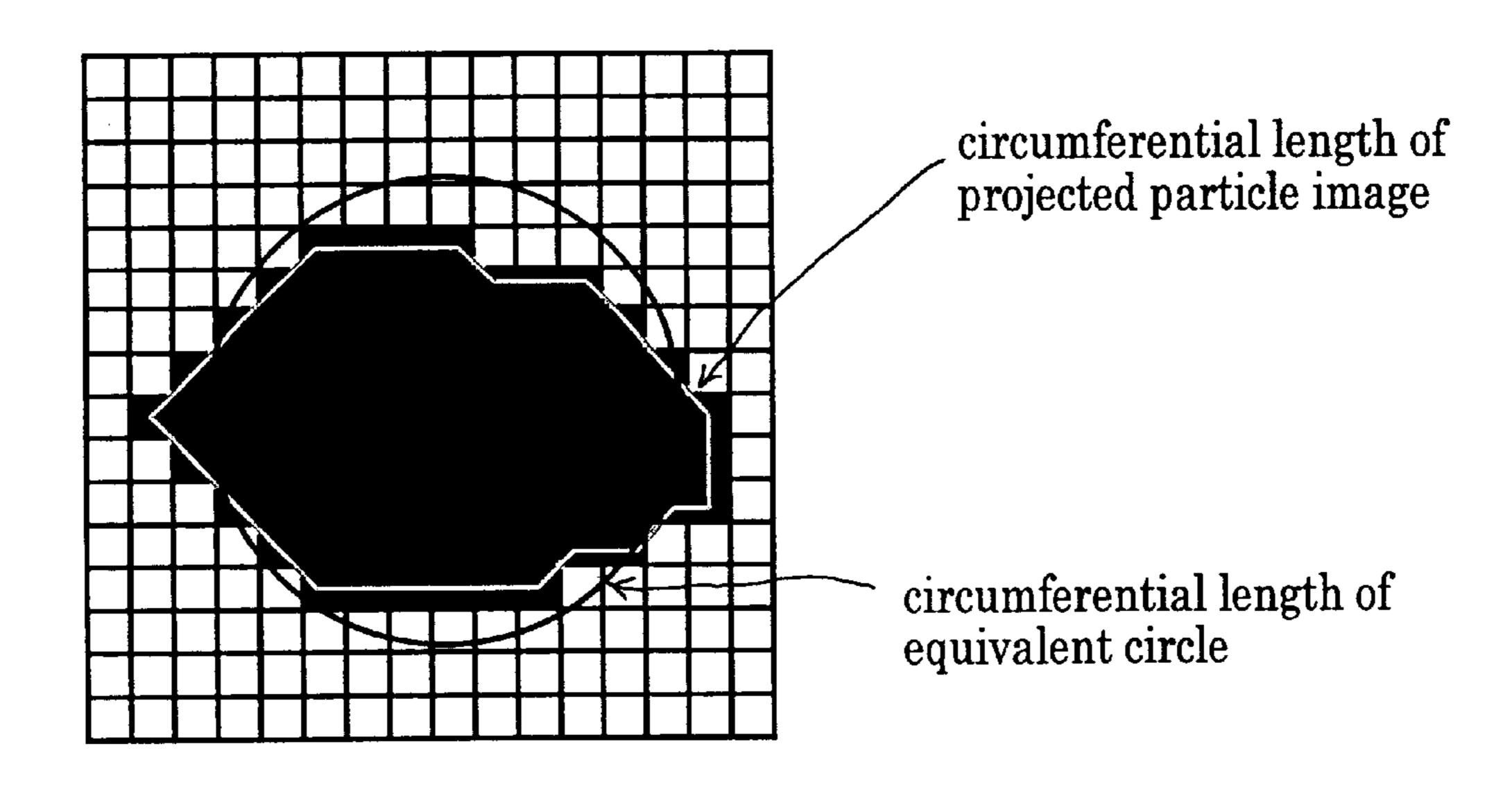
degree of circularity = circumferential length of equivalent circle circumferential length of projected particle image
