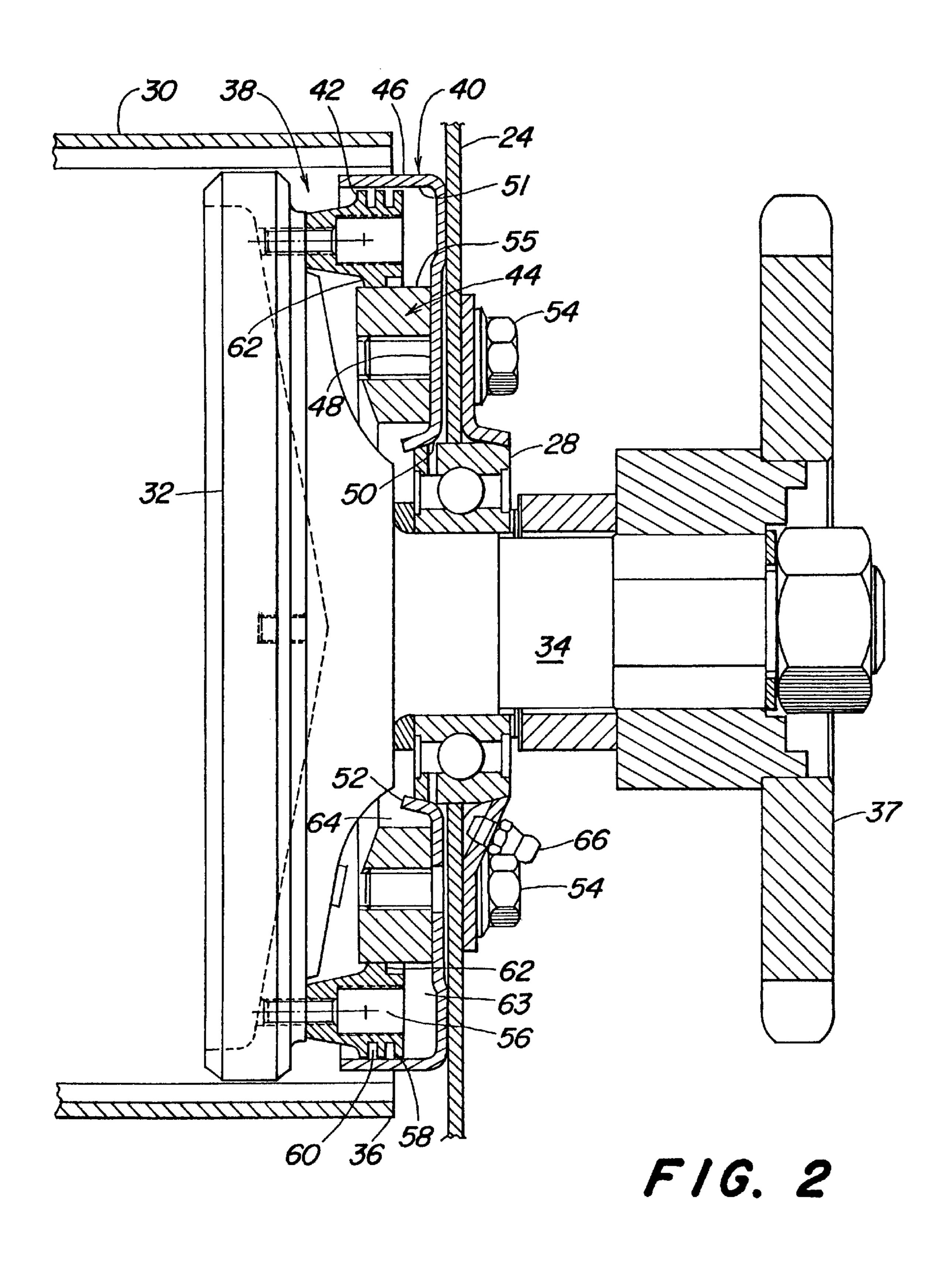
ARRANGEMENT FOR CLOSING A GAP BETWEEN A HARVESTING MACHINE ROLL AND A WALL FOR KEEPING FOREIGN MATTER AWAY FROM A BEARING SUPPORTING A SHAFT OF THE ROLL
