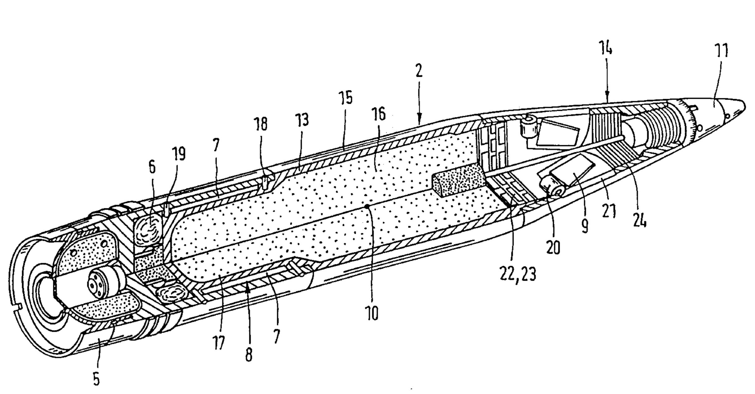
[54] METHOD FOR AUTONOMOUS GUIDANCE OF A SPIN-STABILIZED ARTILLERY PROJECTILE AND AUTONOMOUSLY GUIDED ARTILLERY PROJECTILE FOR REALIZING THIS METHOD
