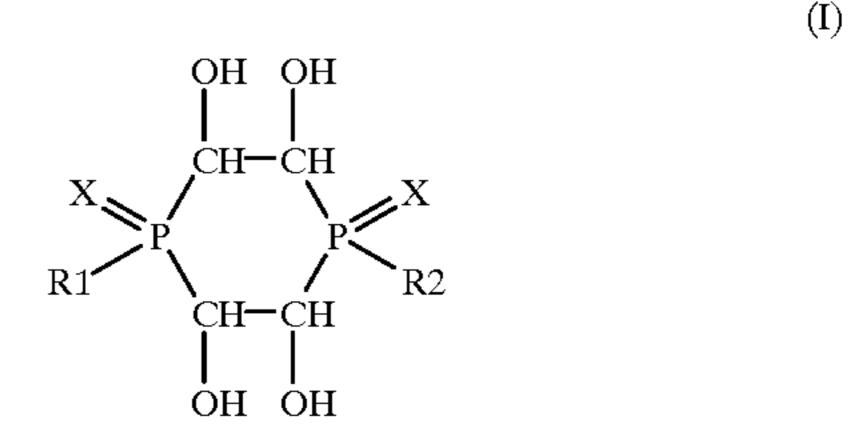
The subject matter of the invention is also the use of compounds of formula I as a flame-retardant agent especially for regenerated celluloses and a process for the flame-retardant finishing of regenerated cellulose which is characterized by mixing in compounds of formula I or a dispersion containing one of these compounds.
