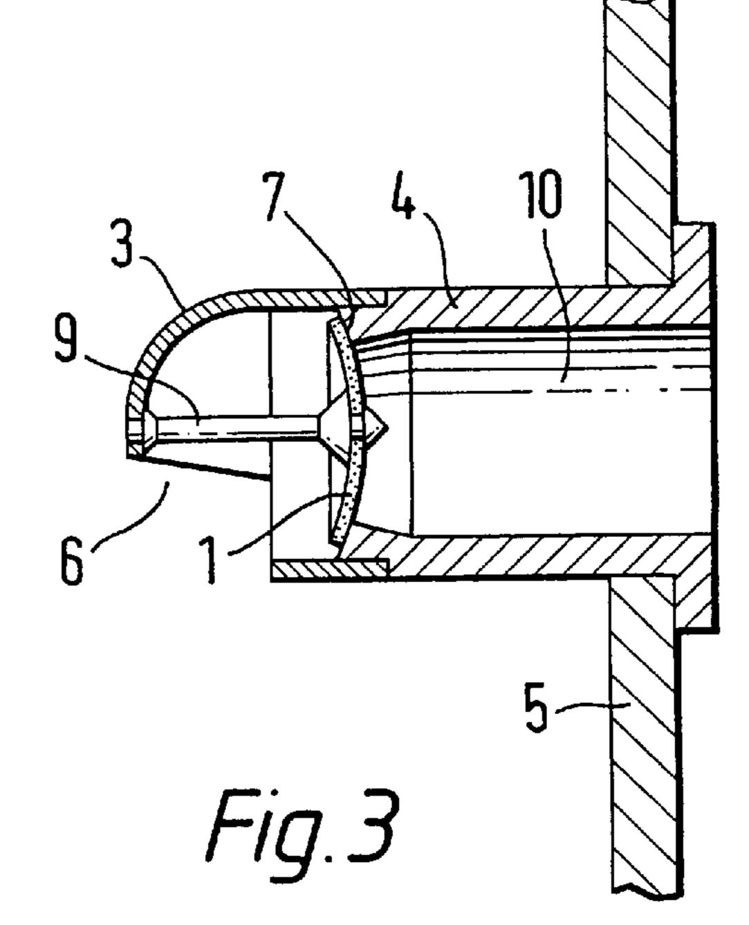
The present invention relates to sealing devices, and more particularly to a device for sealing an opening in a container of a vacuum cleaner or other suction device for 5 collecting dust or other fine material. A preferred embodiment is suitable for picking up and collecting fine toner
