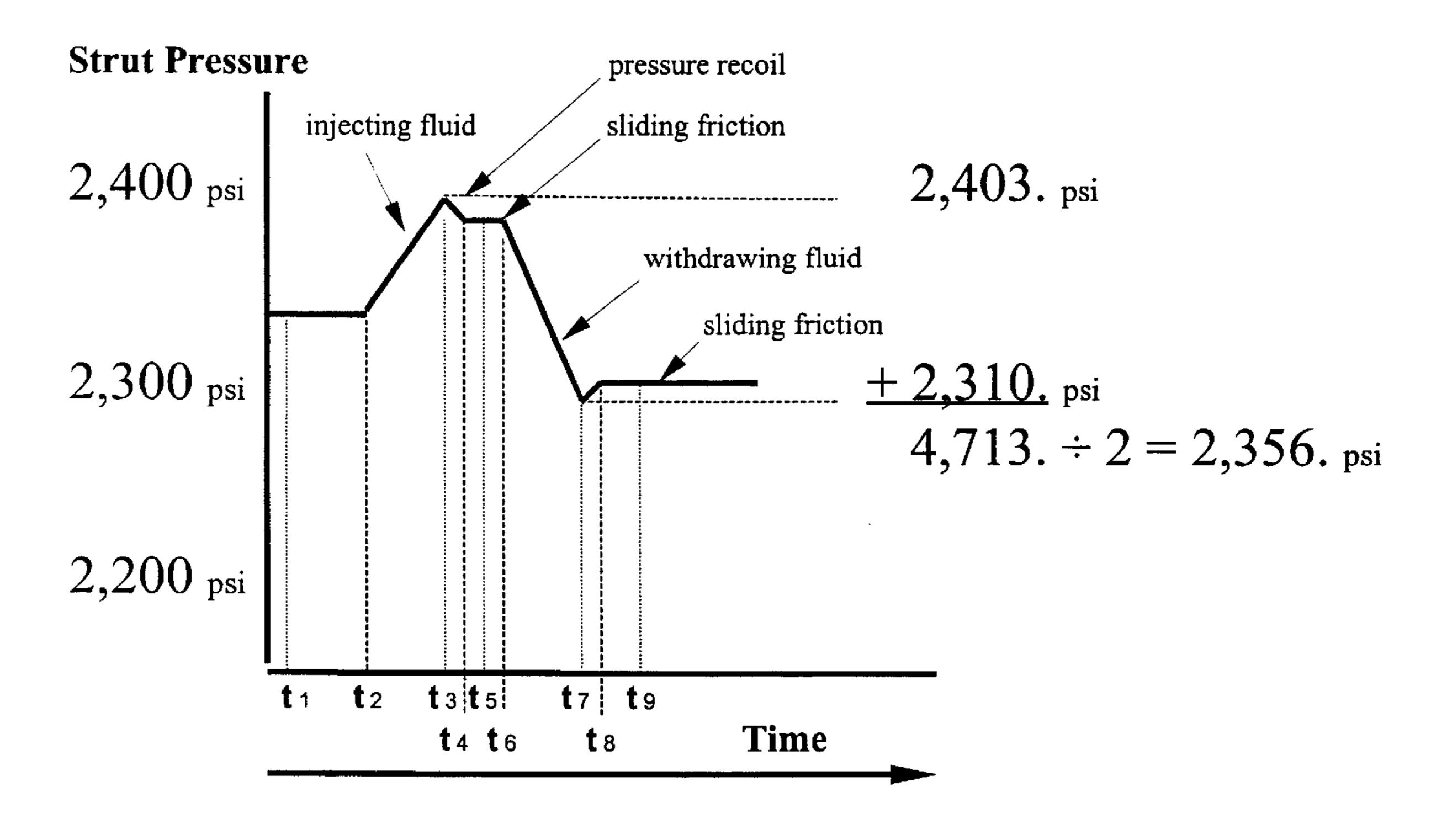
2,356.00 psi 27.34 SQ in (load supporting area within the strut) 64,413.04 lbs sprung weight <u>+ 878.50</u> lbs unsprung weight 65,291.54 lbs supported by left strut 63,812.30 lbs supported by right strut +8.219.78lbs supported by nose strut 137,323.62 lbs - total aircraft weight
