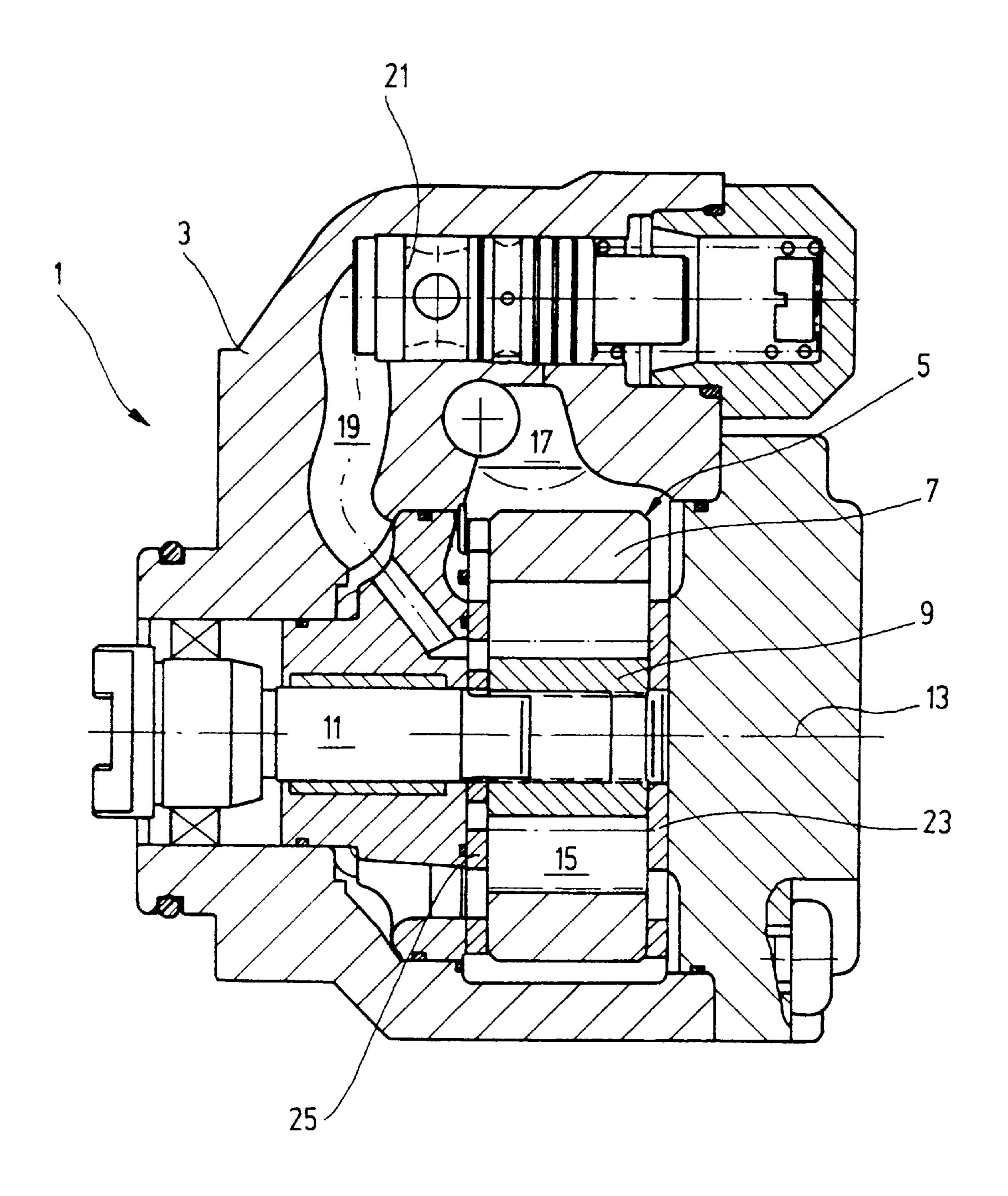
The invention relates to a vane cell pump according to the pre-characterising part of claim 1 and a process of manufacturing a vane cell pump according to the pre- 5 characterising part of claim 4.
