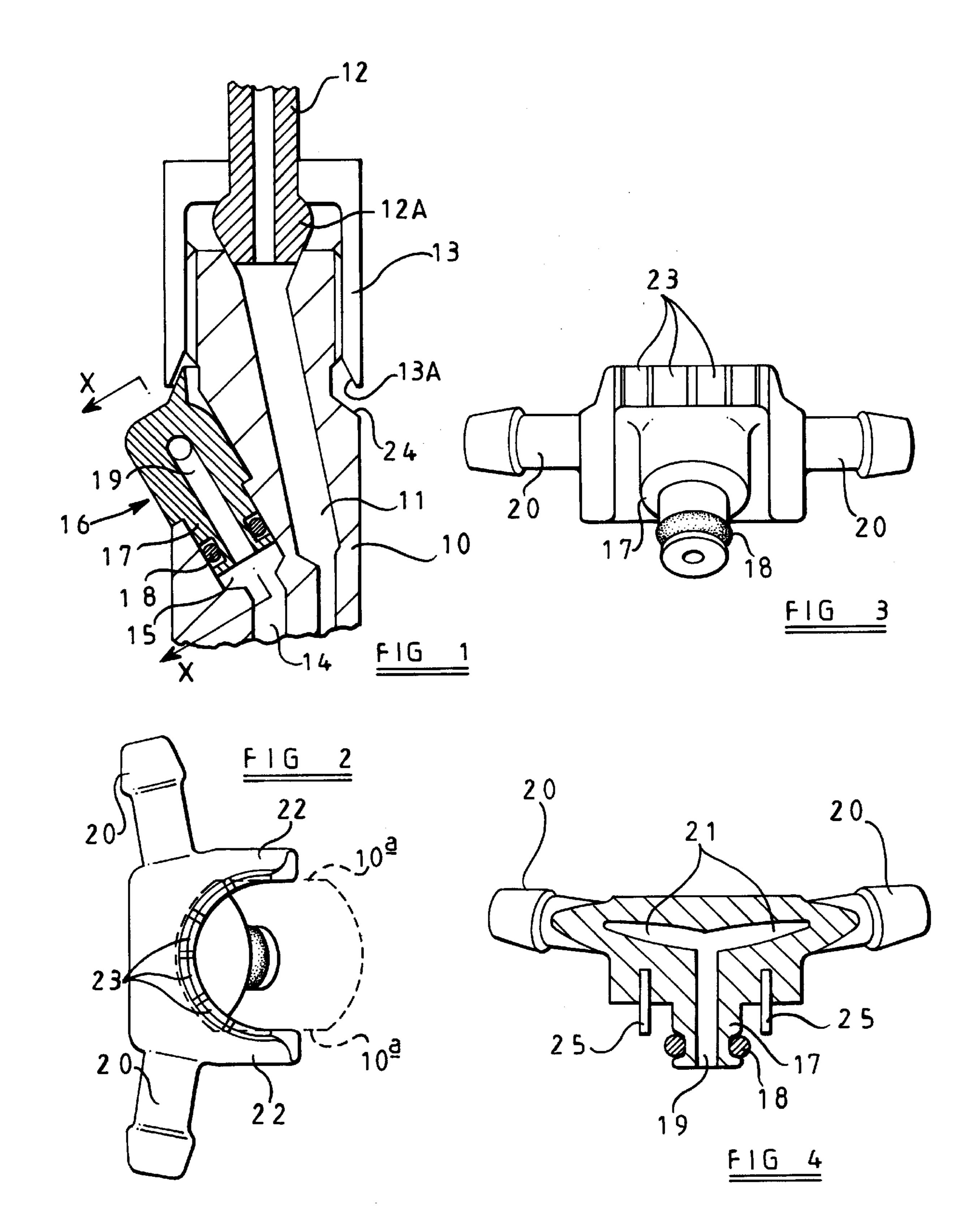
This invention relates to a connector for use in the return of fuel from an injector to a suitable low pressure fuel reservoir.
