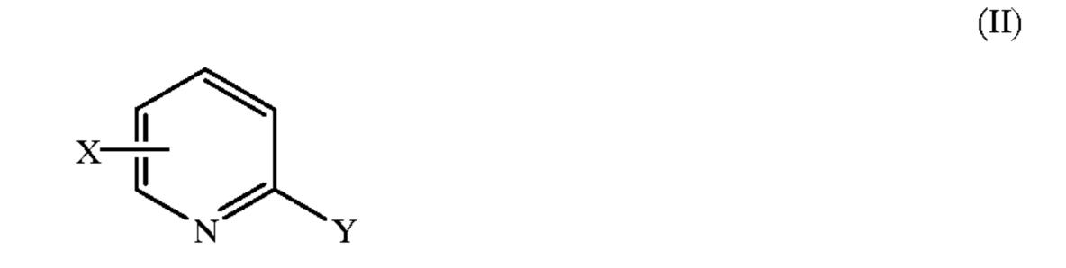
wherein X and Y each independently represents a halogen atom [hereafter abbreviated halogenopyridine derivatives (II)], which comprises reacting a halogeno-2sulfonylpyridine represented by the general formula (I):
