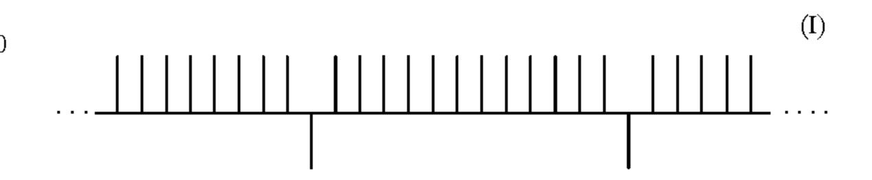
Isotactic polypropylene is capable of forming a highly crystalline polymer with crystalline melting points and other desirable physical properties that are considerably different from the same polymer in an amorphous, or noncrystalline, state.
