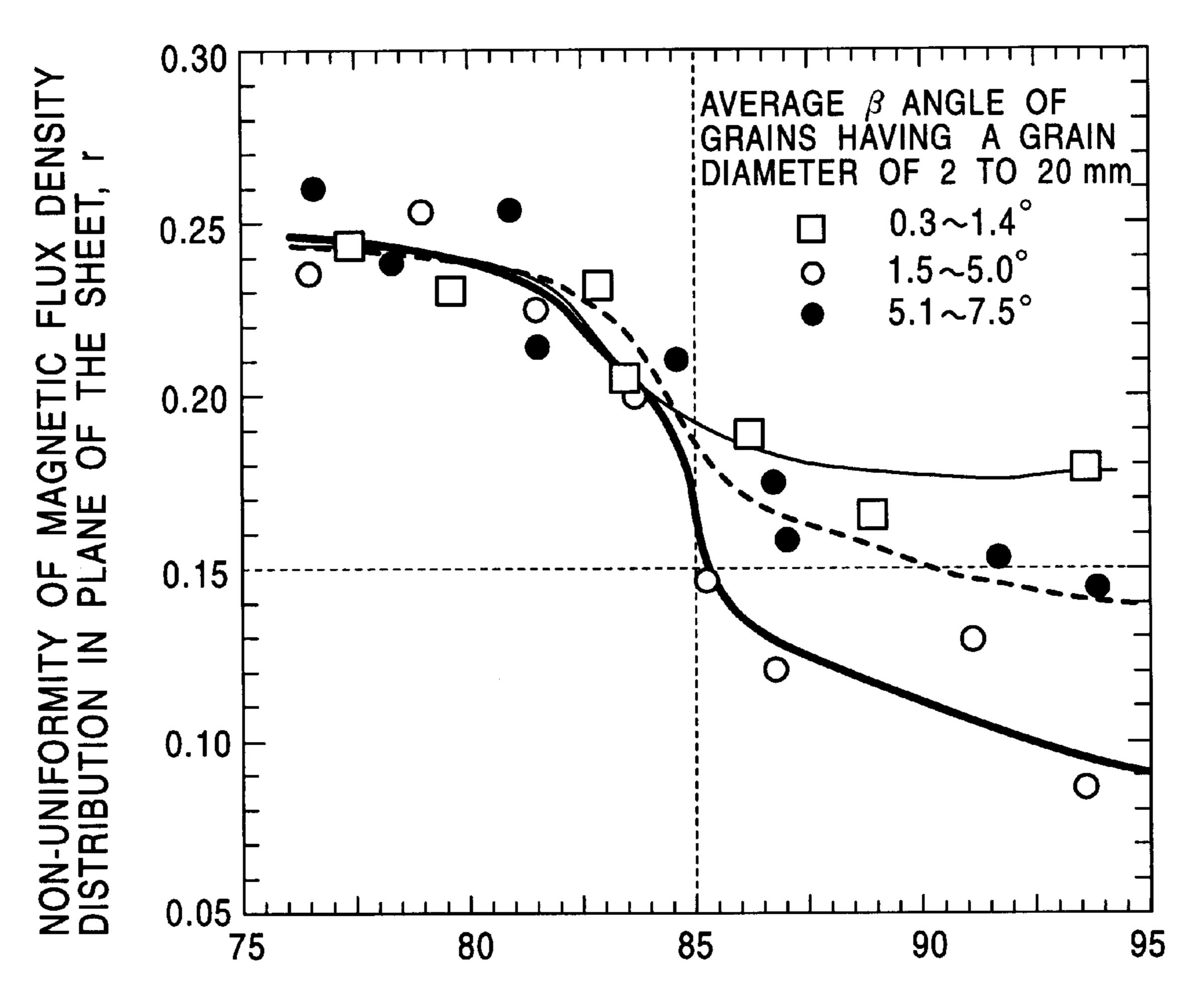
PROPORTION (%) OF SECONDARY RECRYSTALLIZED GRAINS HAVING A MAXIMUM LENGTH OF 60 mm OR MORE IN DIRECTION PERPENDICULAR TO ROLLING
