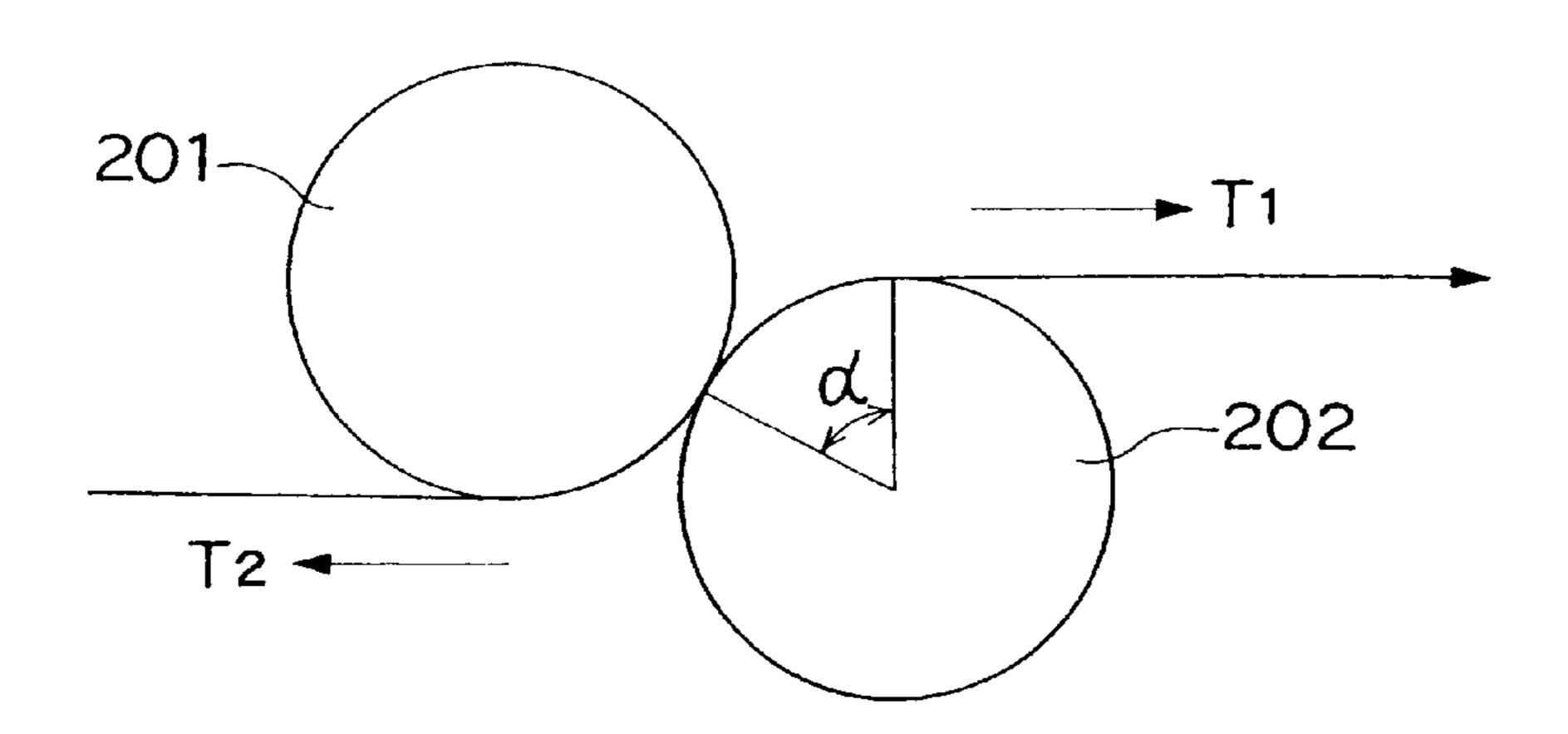
TRANSMISSION TORQUE  $T = rTe(e^{\mu \alpha}-1)/e^{\mu \alpha}$ EFFECTIVE TENSION  $Te = T_1 - T_2$
