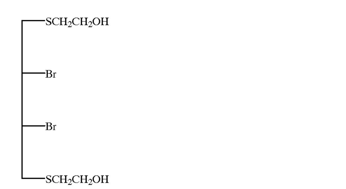
Then, 257.9 g (1.5 moles) of 47' hydrobromic acid and 190.3 g (2.5 moles) of thiourea were added to the viscous liquid. The mixture was subjected to isothiouronium salt reaction, hydrolysis, purification and removal in the same manner as in Example 3 to obtain 131.7 g (0.429 mole; yield 85.8%) of the following polythiol FSH2, the same polythiol as obtained in Example 3, as a colorless, transparent and viscous liquid.
