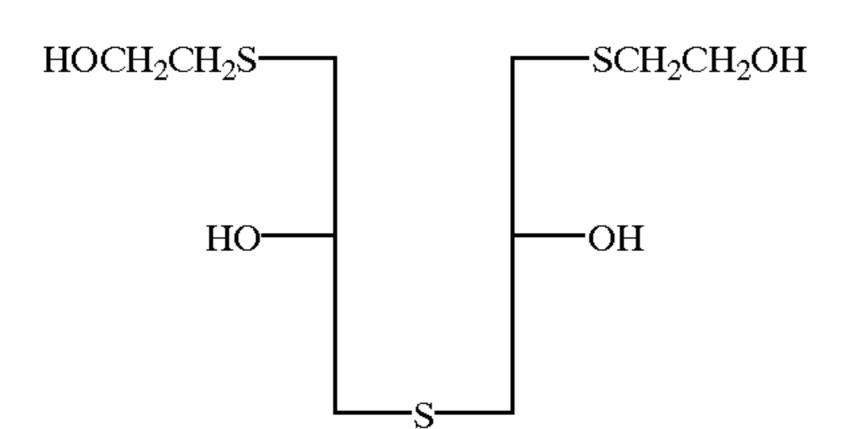
Then, 303.8 g (3.0 moles) of 36% hydrochloric acid and 190.3 g (2.5 moles) of thiourea were added to the reaction liquid and the mixture was heated at 110° C. for 9 hours under stirring.
