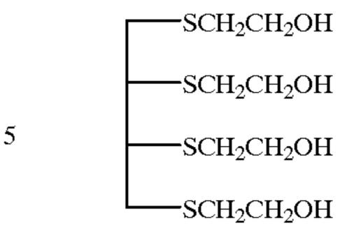
Then, 253.2 g (2.5 moles) of 36% hydrochloric acid and 152.2 g (2.0 moles) of thiourea were added to the viscous liquid. The mixture was subjected to isothiouronium salt reaction, hydrolysis, purification and removal in the same manner as in Example 3 to obtain 205.0 g (0.480 mole; yield 96.0%) of the following polythiol FSH5, as a colorless, transparent and viscous liquid.
