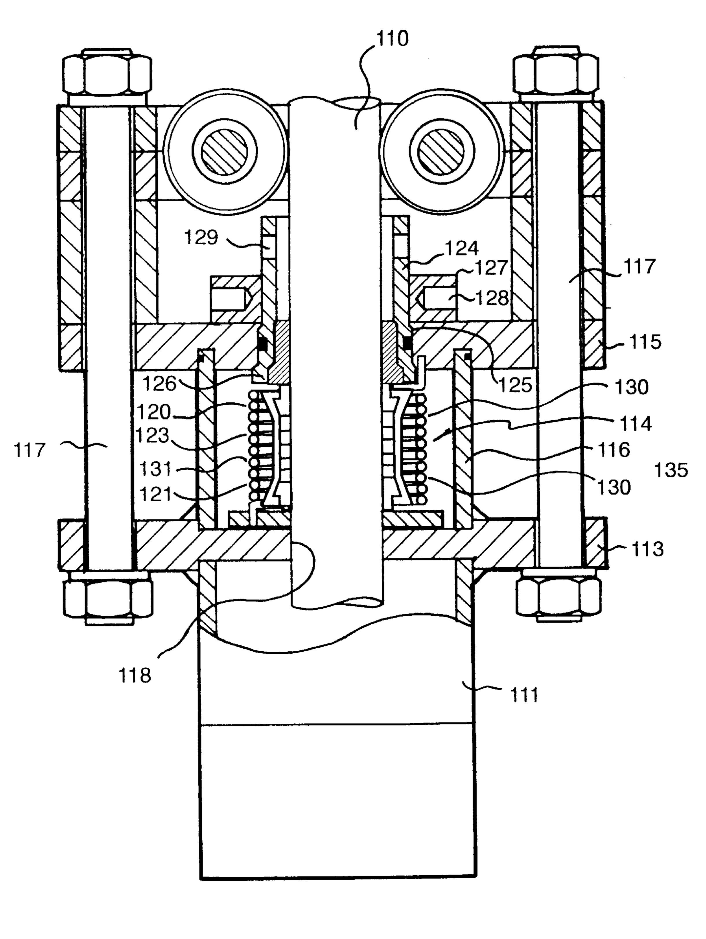
THIS INVENTION relates to a seal and in particular relates to a seal which is to be used in providing sealing engagement between two members which are capable of 5 relative movement with respect to each other.
