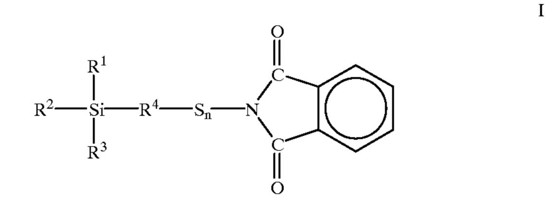
wherein R<sup>1</sup>, R<sup>2</sup> and R<sup>3</sup> are independently selected from the group consisting of alkoxy radicals having from 1 to 8 carbon atoms; R<sup>4</sup> is selected from the group consisting of alkylene groups having from 1 to 15 carbon atoms and arylene and alkyl substituted arylene groups having from 6 to 10 carbon atoms; and n is an integer of from 1 to 8.
