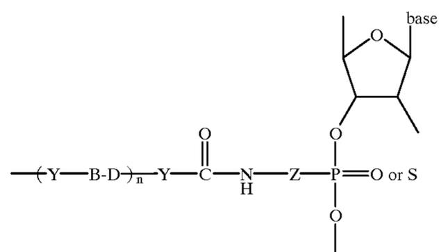
In a preferred embodiment, the conductive oligomer is covalently attached to the nucleic acid via a transition metal ligand. In this embodiment, the conductive oligomer is covalently attached to a ligand which provides one or more of the coordination atoms for a transition metal. In one embodiment, the ligand to which the conductive oligomer is
