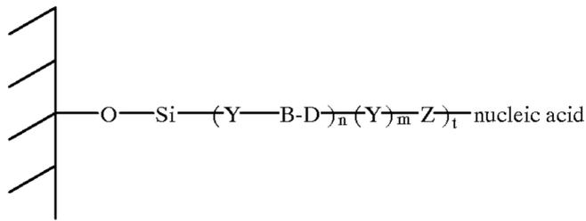
In Structure 29, the oxygen atom is from the oxide of the metal oxide electrode. The Si atom may also contain other atoms, i.e. be a silicon moiety containing substitution groups.
