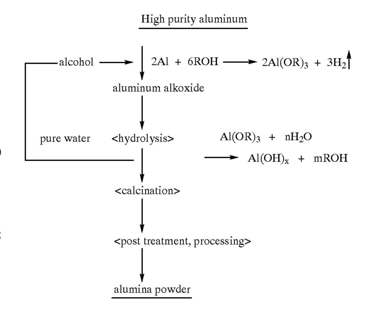
In the above-process, metallic aluminum is reacted with an alcohol, such as methanol, to form an alkoxide, which is then hydrolyzed to provide aluminum hydroxide. The aluminum hydroxide is then calcined to obtain powdery alumina.
