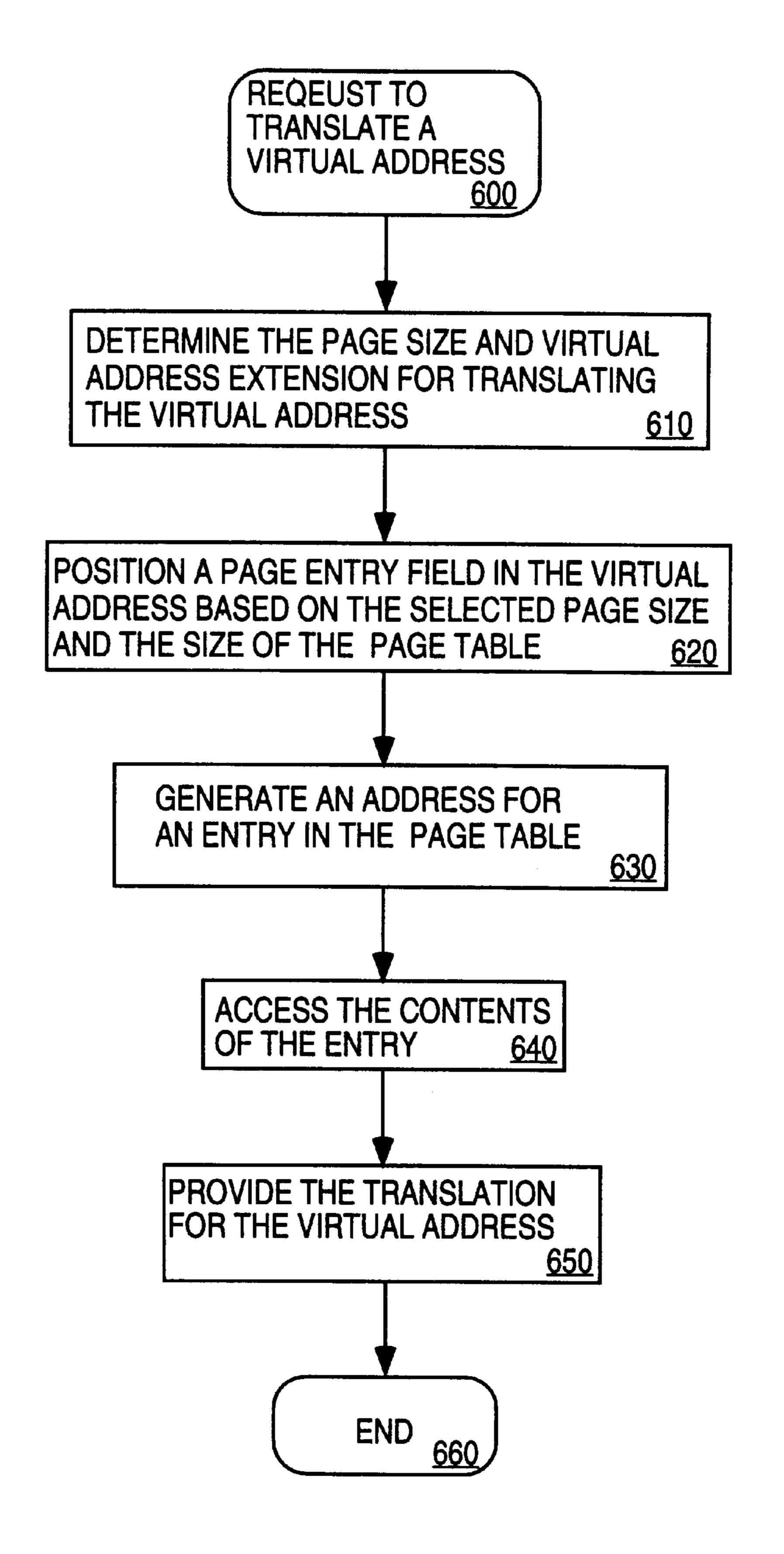
PAGE TABLE WALKER THAT USES AT LEAST ONE OF A DEFAULT PAGE SIZE AND A PAGE SIZE SELECTED FOR A VIRTUAL ADDRESS SPACE TO POSITION A SLIDING FIELD IN A VIRTUAL ADDRESS
