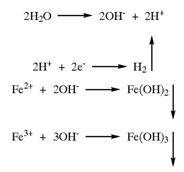
The developing hydrogen gas adheres to ferro- and ferrihydroxide deposits, which are in turn producing a web or mesh structure for trapping solid impurities. This way, the solid matter flocculates and the flock-adhered hydrogen gas makes the flock lighter than water.
