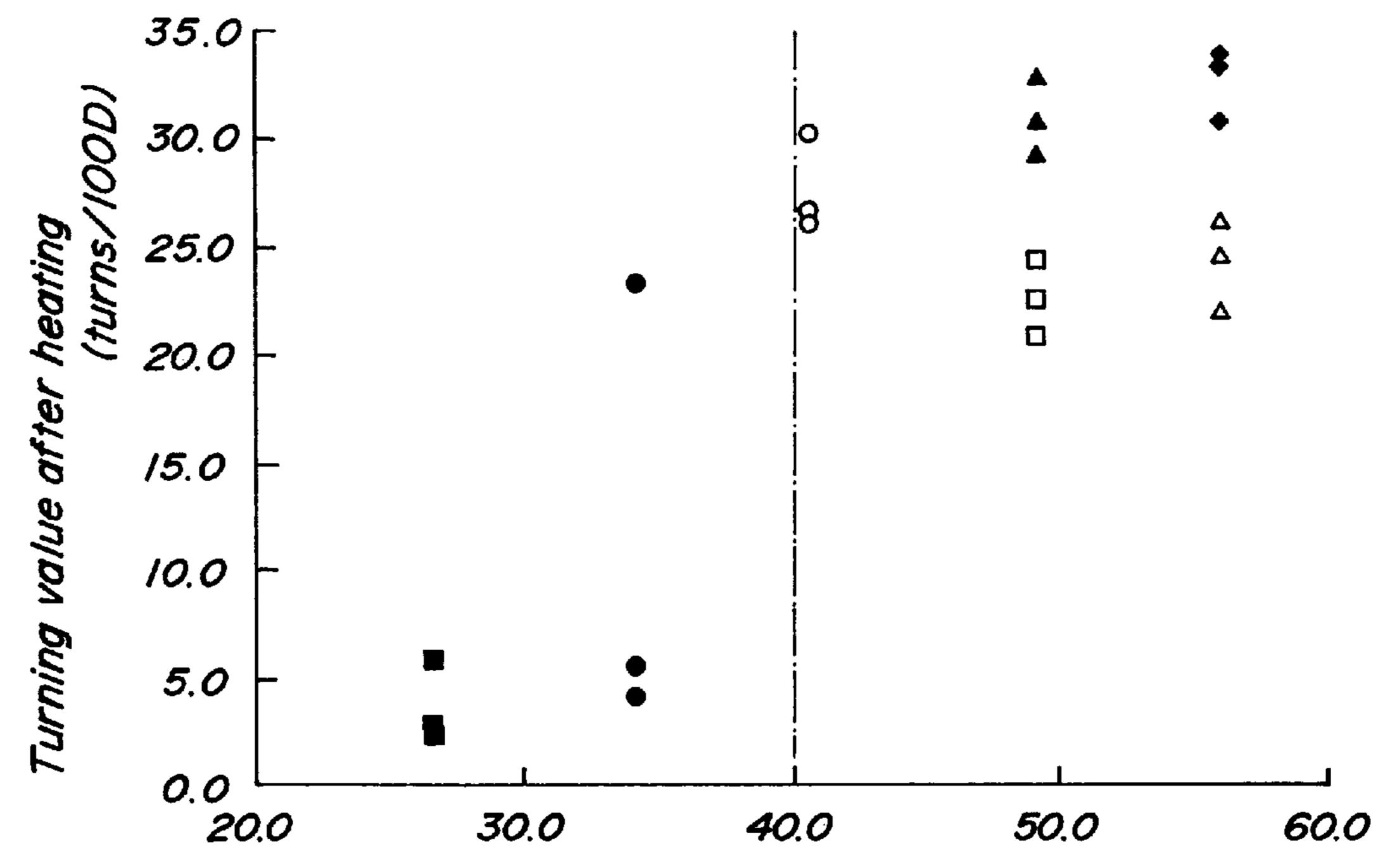
Ratio of wire drawing through die having reduction of area of not less than 20% (%)
