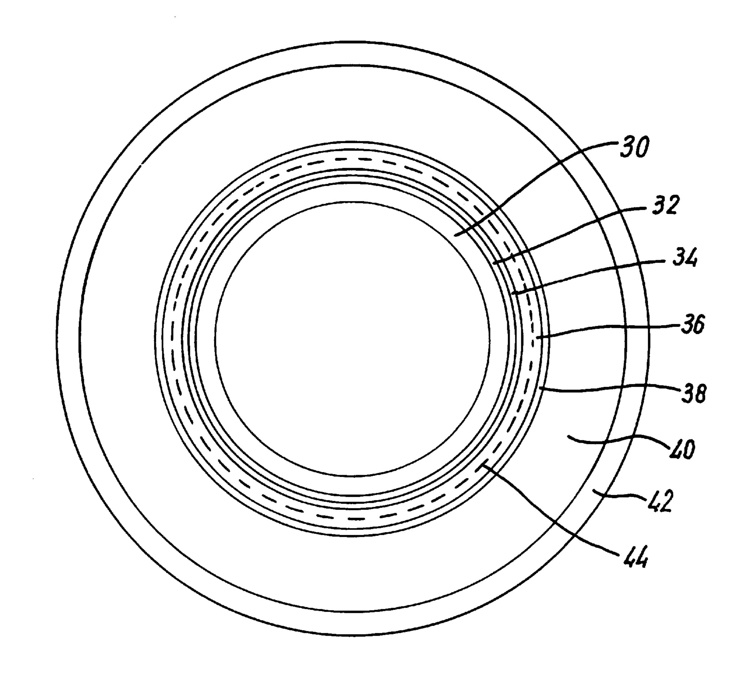
This invention relates to the coating of pipelines and the like, particularly subsea pipelines and risers, but also other forms of ducting and piping, for the purpose of providing 5 thermal insulation. The invention provides an improved coating method and an improved coated pipeline formed thereby.
