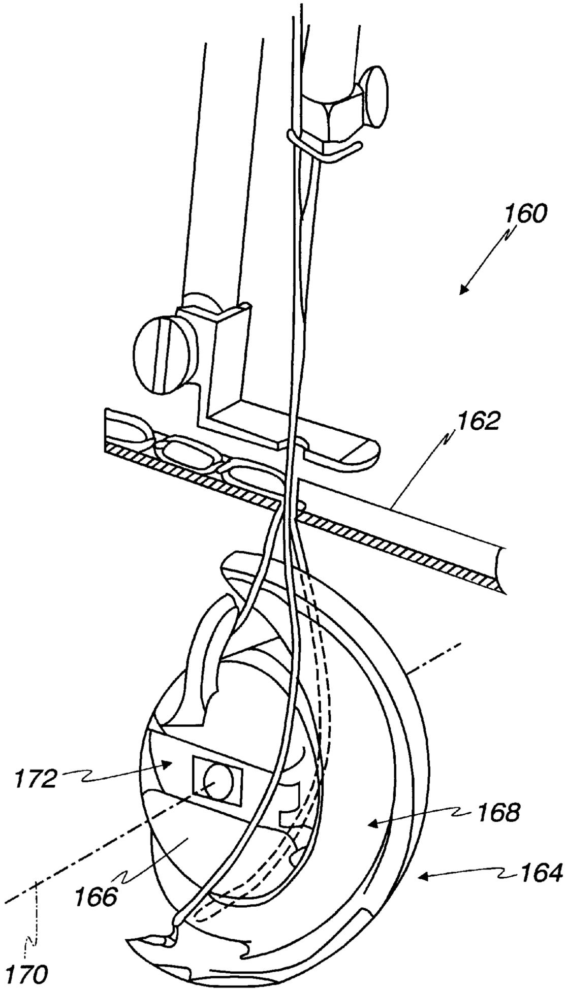
**HOOK SYSTEM FOR SEWING MACHINE****FIELD OF THE INVENTION**
