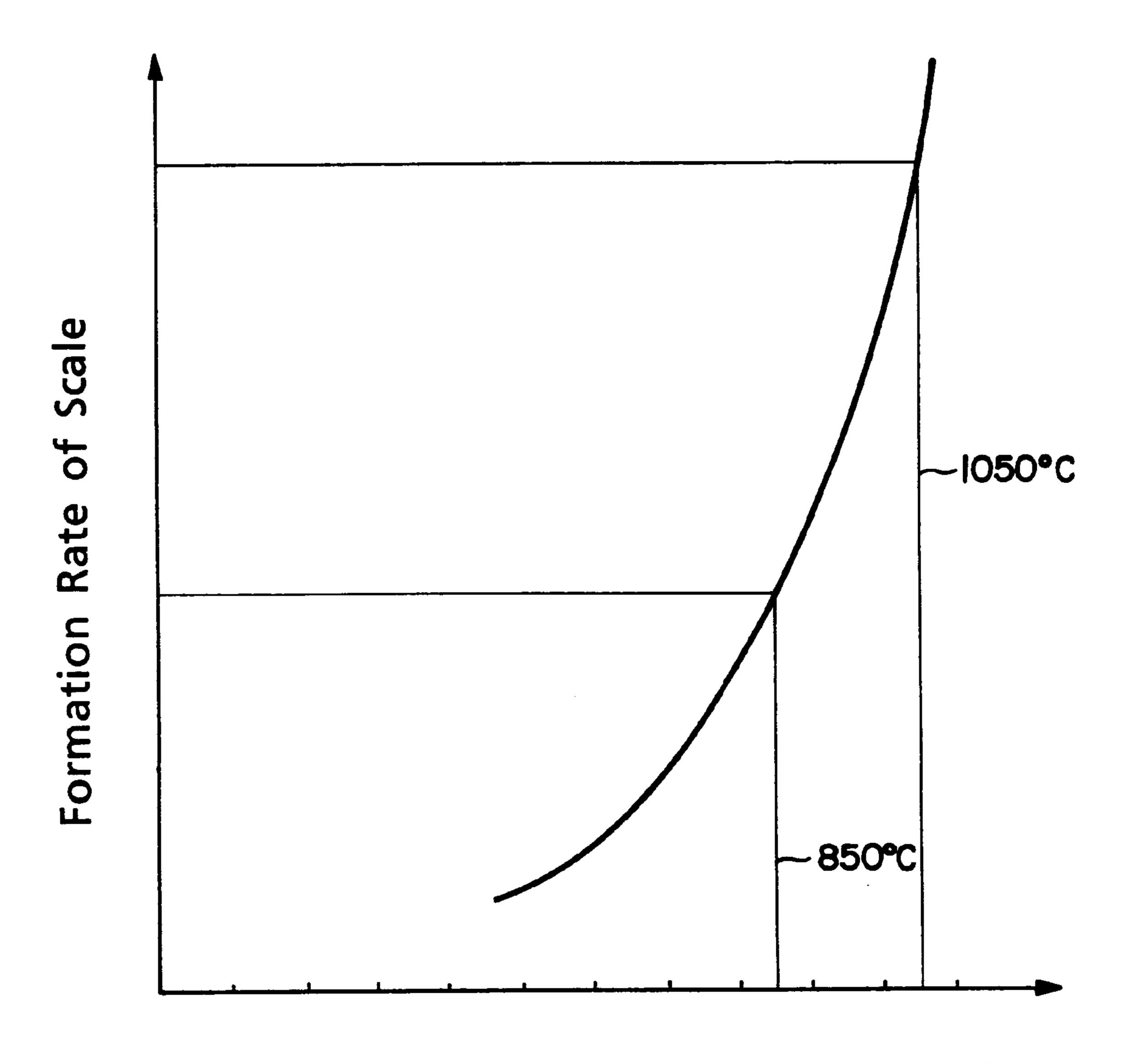
Surface Temperature of Rolled Material
