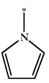
wherein the pyrrole ring shown may be substituted or unsubstituted, and \* represents the position of bonding to the benzo ring shown in formula (III).
