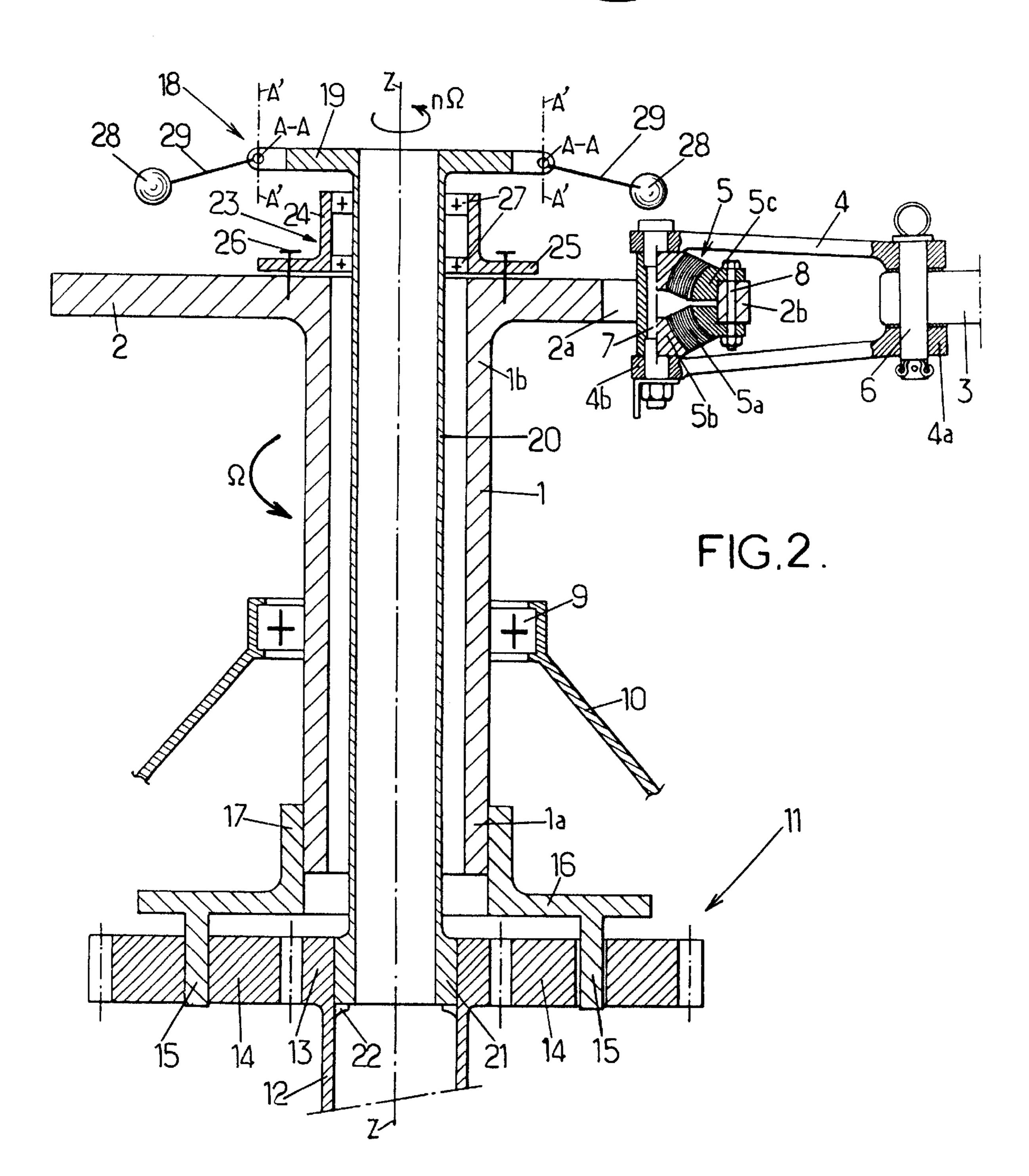
The invention concerns rotor head resonators, in particular those for the main rotor on a helicopter. These are the devices for attenuating the vibrations generated by the 5 rotational motion of a rotor, the resonators being used at the position of the rotor heads in order to counter the vibrations effectively, directly at their source of production.
