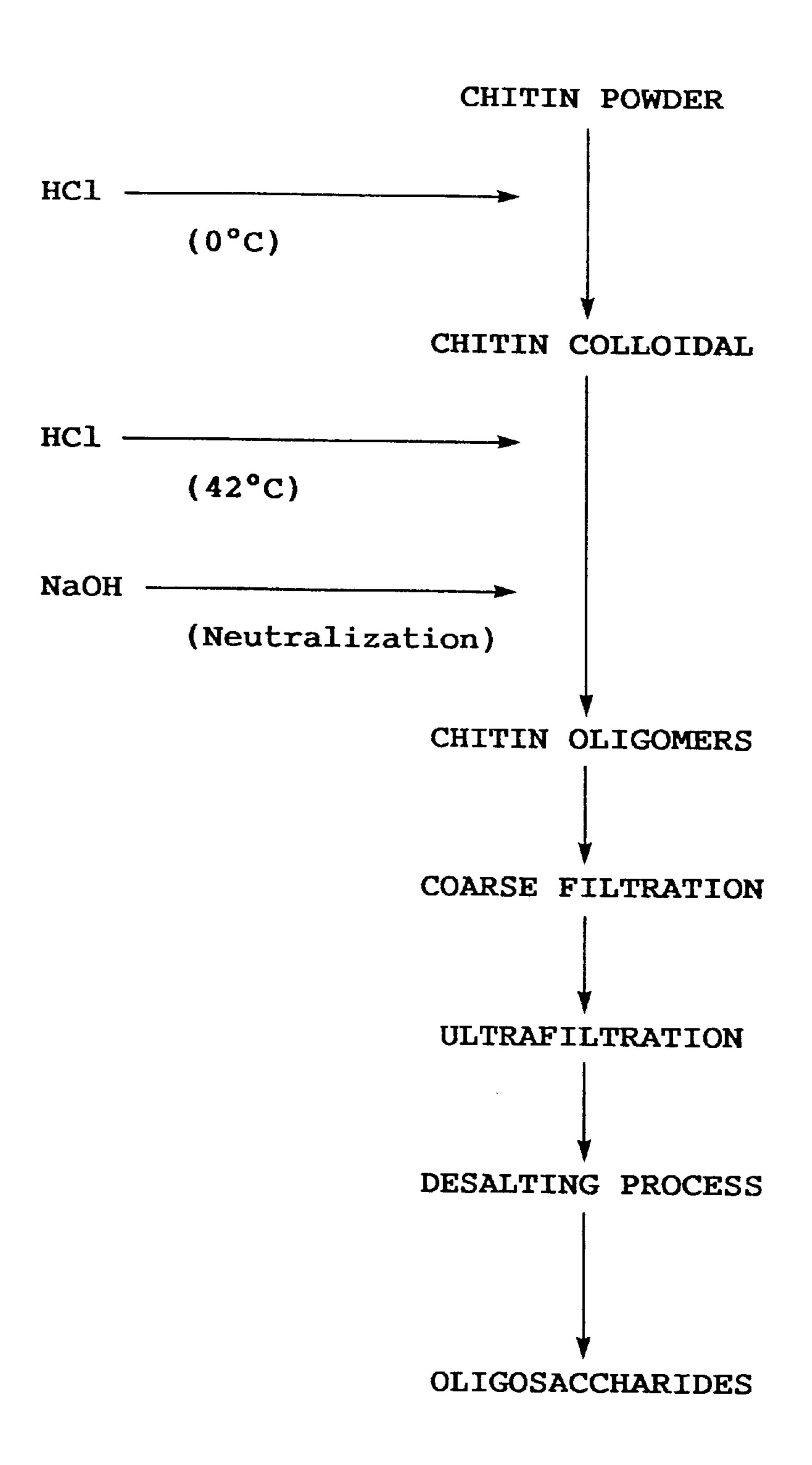
Fig. 1 Flowchart of preparation chitin oligomers.
