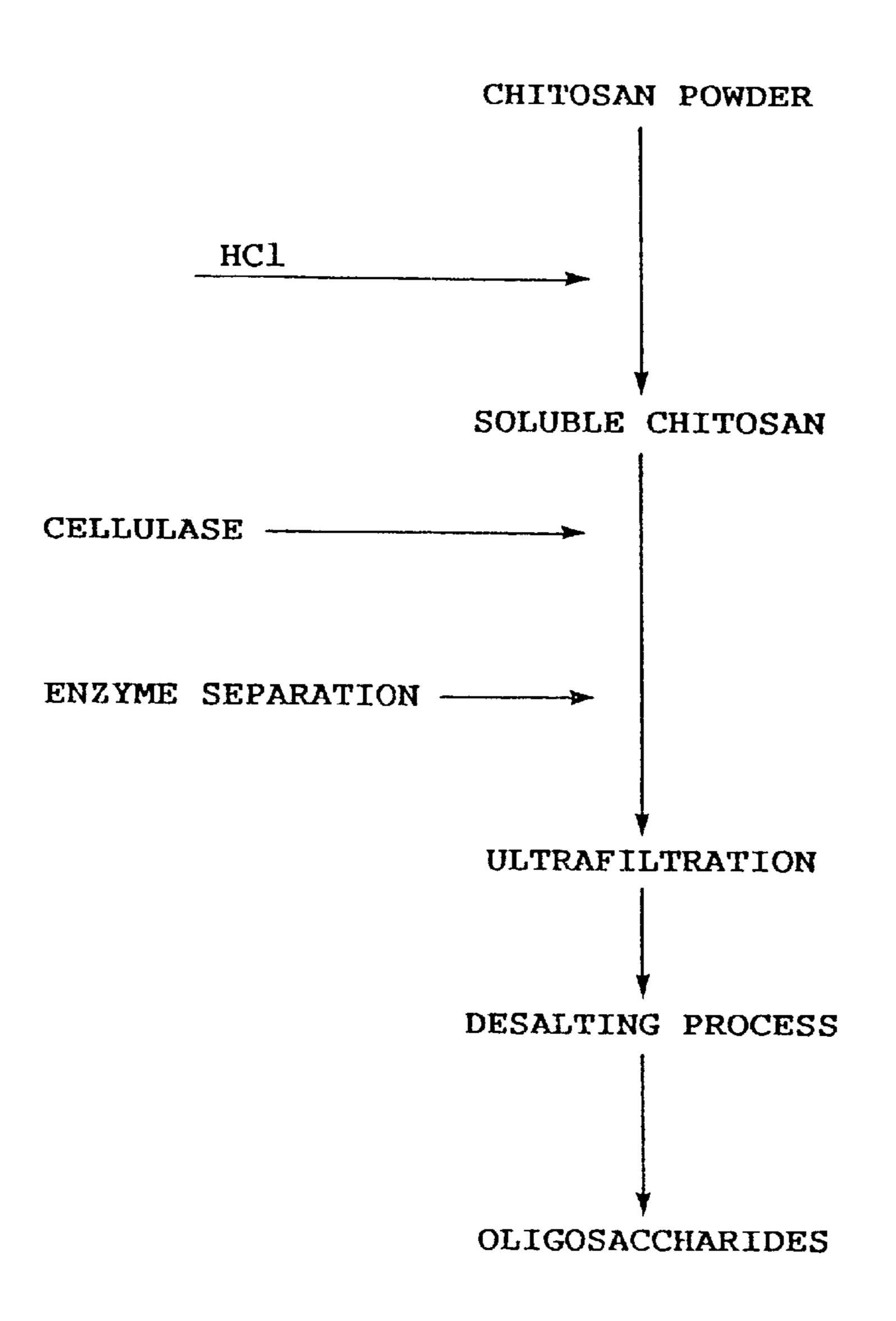
Fig. 2 Flowchart of preparation chitosan oligomers.
