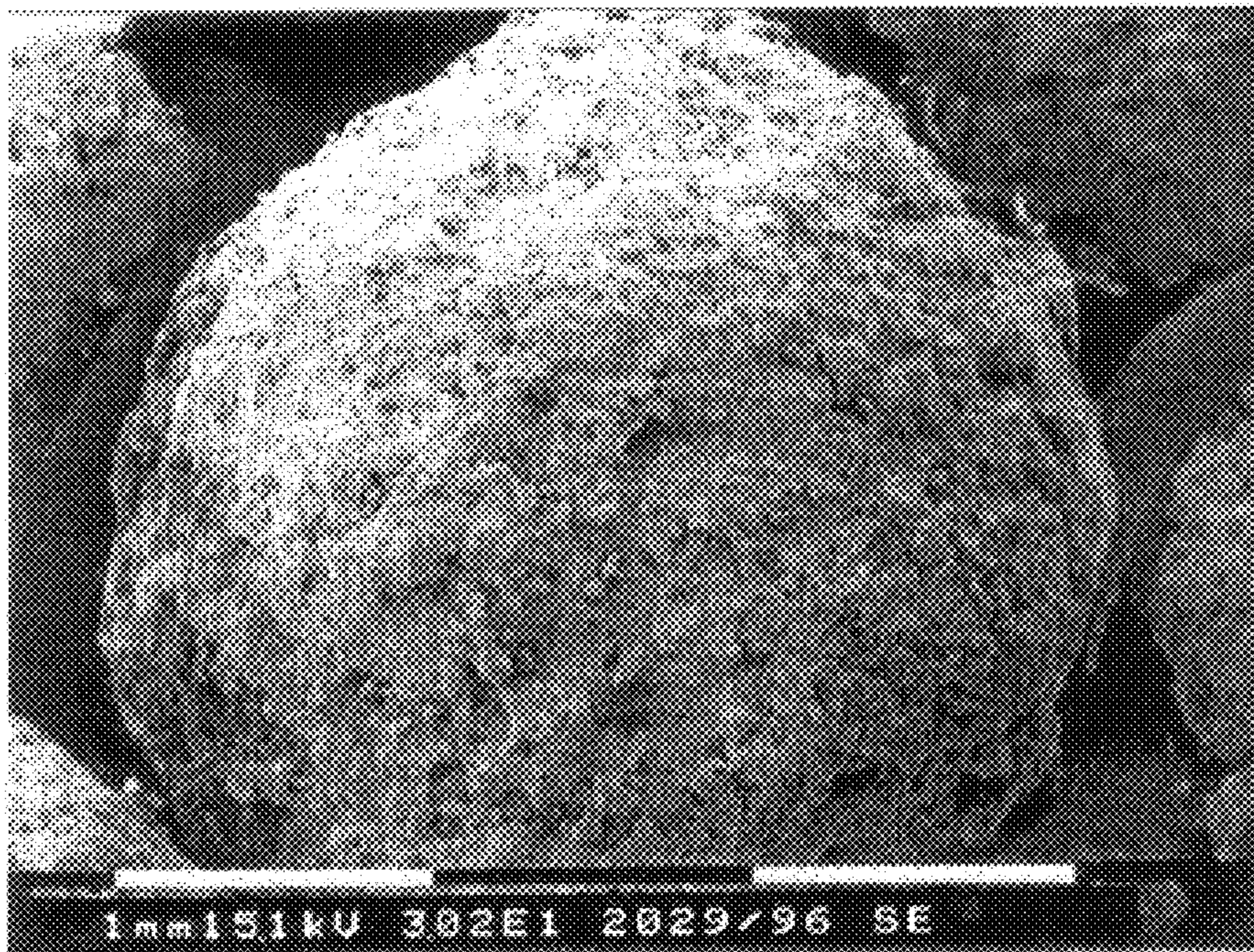
SEM picture of a porous polyolefin particle, magnification 30x
