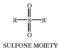
Examples of sulfone polymers are polysulfone, polyethersulfone, and polyarylsulfone. A hydrophilic second polymer is utilized in addition to the hydrophobic polymer. Preferably, the second polymer is polyvinylpyrrolidone. It may also be a co-polymer derivative of polyvinylpyrrolidone, such as a polyvinylpyrrolidone/polyvinylacetate co-polymer.
