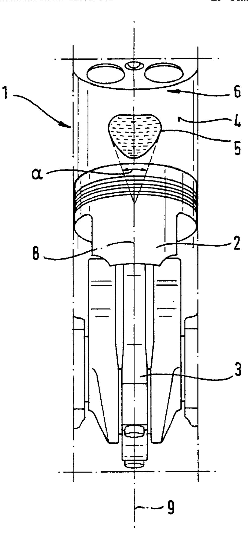
[54] WEAR RESISTANT CYLINDER BARREL SURFACE FOR SUPPORTING A PISTON
