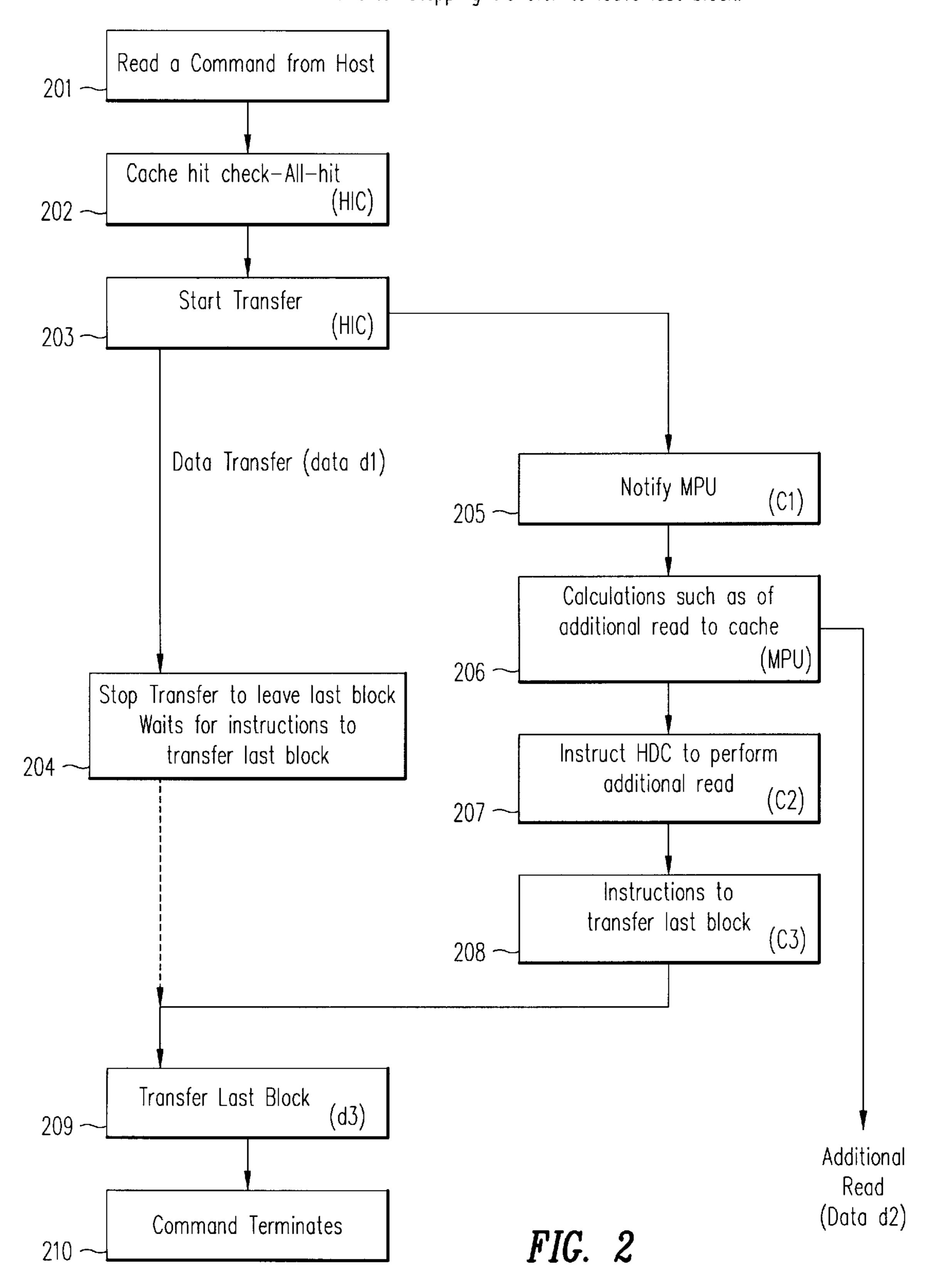
Case in which instructions on transfer of last block are received from local MPU before stopping transfer to leave last block.
