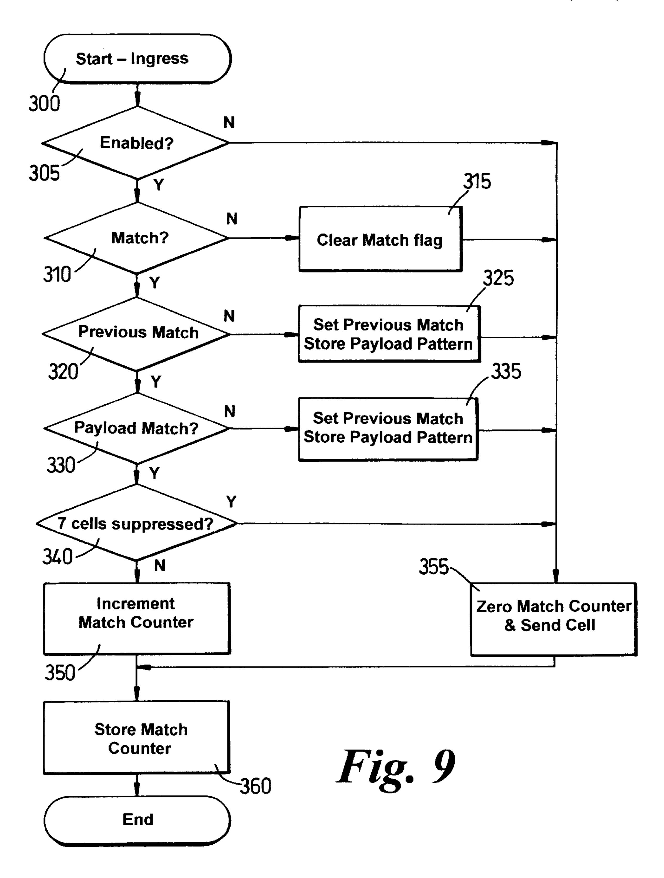
Match = All bytes in payload are identical Previous Match = Previous cell had all bytes in payload identical Payload Match = New cells payload matches the payload of the previous cell
