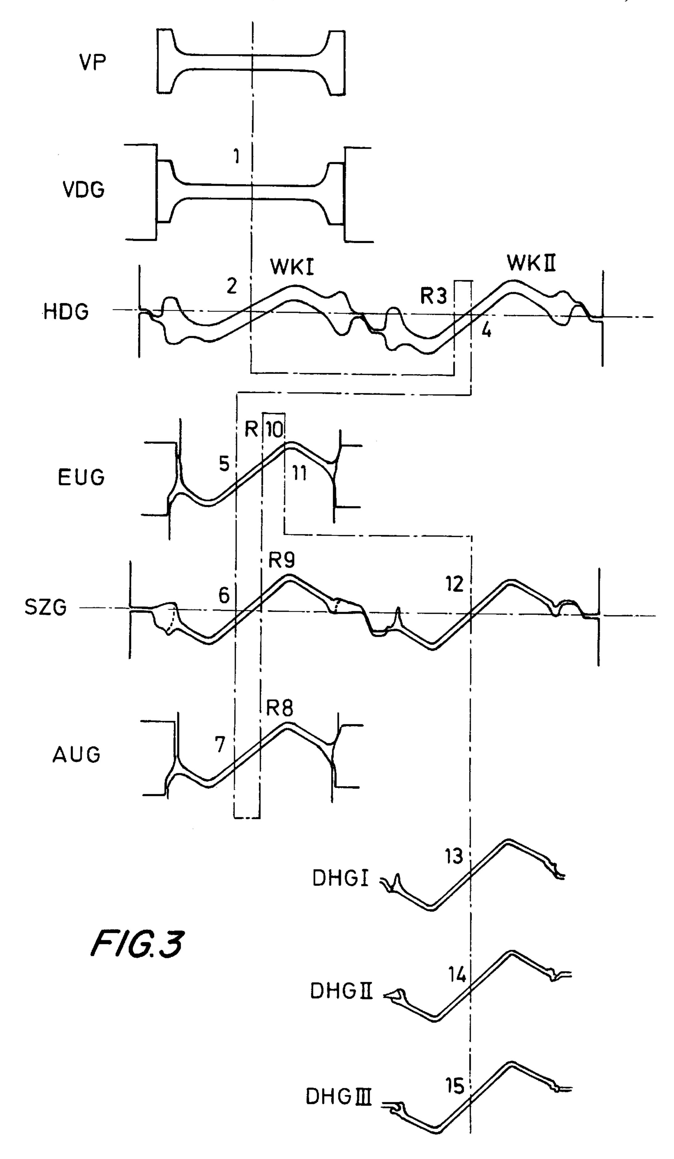
METHOD OF CASTING AND ROLLING AND ROLL STAND ARRANGEMENT FOR ROLLING FINISHED SECTIONS (SHEET PILING SECTIONS) FROM A PRELIMINARY SECTION ARRIVING FROM A CONTINUOUS CASTING MACHINE AND HAVING APPROXIMATE FINAL **DIMENSIONS**
