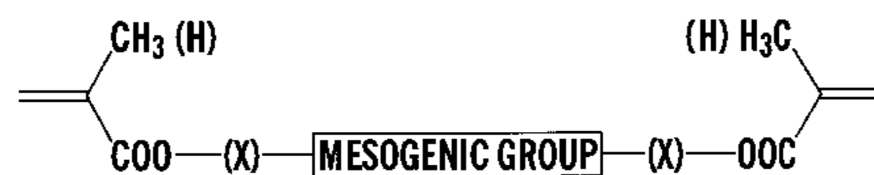
TERMINAL ARRANGEMENT OF THE METHACRYLIC OR ACRYLIC GROUPS
