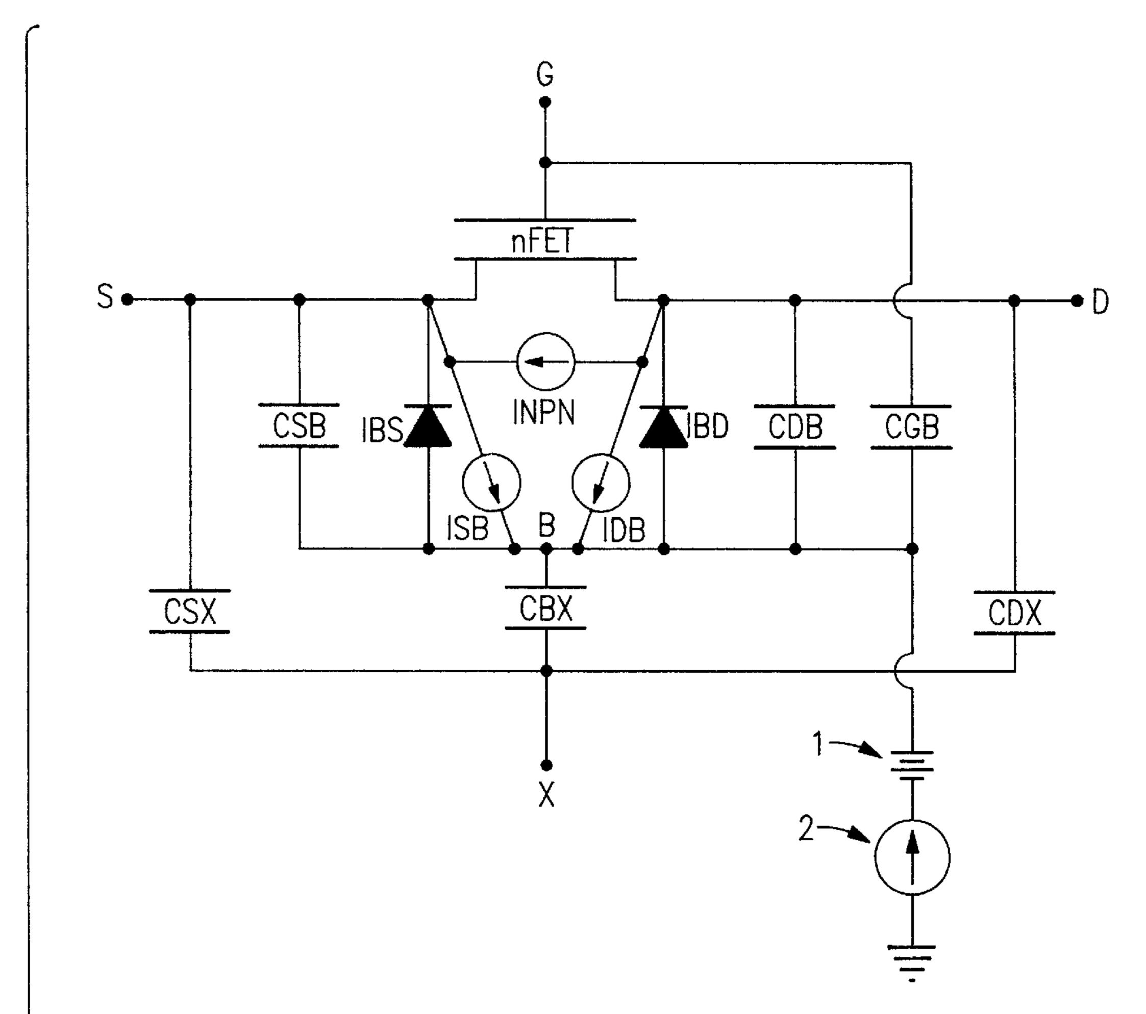
INPN PARASITIC LATERAL NPN TRANSISTOR COLLECTOR CURRRENT IBS, IBD INTERNAL BASE—EMITTER AND BASE—COLLECTOR DIODES FOR NPN ISB, IDB IMPACT IONIZATION CURRENT WHICH CHARGES FLOATING BODY CSB, CDB THESE CAPACITORS INCLUDE EXTRA DIFFUSION CAPACITANCE CSX, CBX, CDX CAPACITANCE TO BACK OXIDE INTERNAL FLOATING BODY NODE
