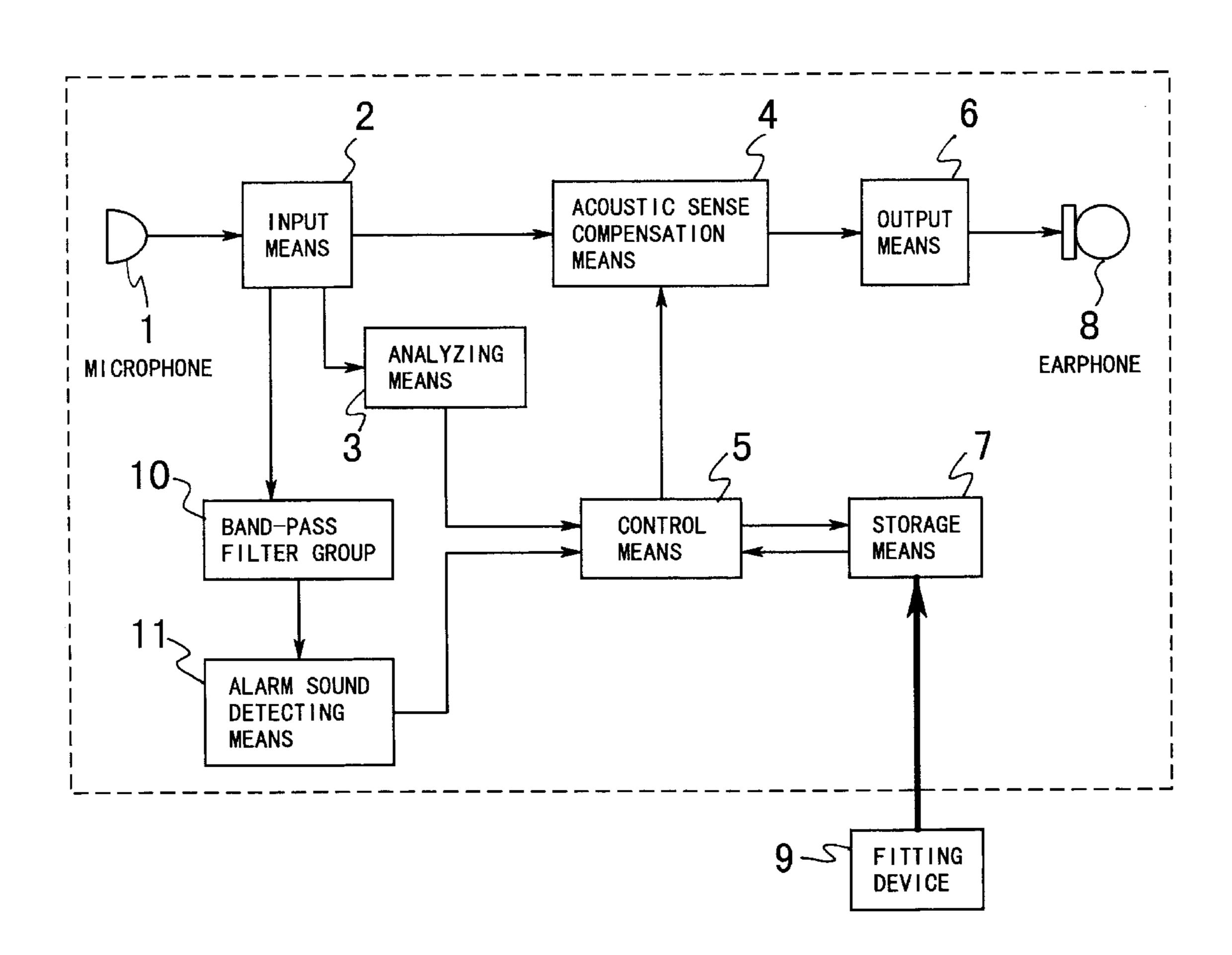
9 FITTING DEVICE STORAGE Means OUTPUT MEANS 4 ACOUSTIC SENSE COMPENSATION MEANS  $\mathbf{C}$ CONTROL YZING ANALY. MEANS -PASS ER GROUP S I NPUT MEANS ALARM DETECT MEANS MICROPHONE
