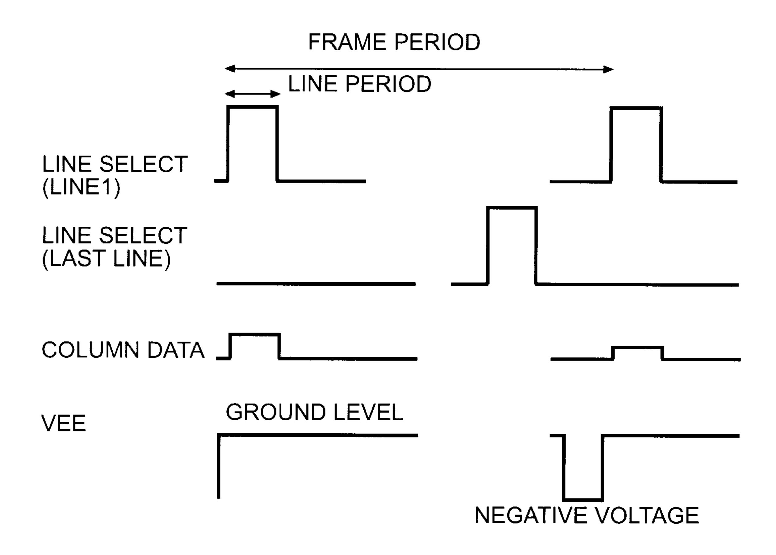
NOTE:COLUMN DATA IS SHOWN AT DIFFERENT LEVELS TO REPRESENT DIFFERENT INFORMATION (AMPLITUDE MODULATION)
