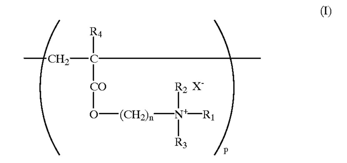
wherein R<sub>1</sub> is an aralkyl group having from 7 to 10 carbon atoms or An alkyl group having from 1–20 carbon atoms; R<sub>2</sub> and R<sub>3</sub> are each independently the same or different and represent a lower alkyl group having from 1-4 carbon atoms; R<sub>4</sub> is a hydrogen atom or a lower alkyl group having 1–4 carbon atoms; X is a physiologically acceptable counter ion; n is an integer of from 1 to 3; and p is an average degree of polymerization of from 10 to 10,000.
