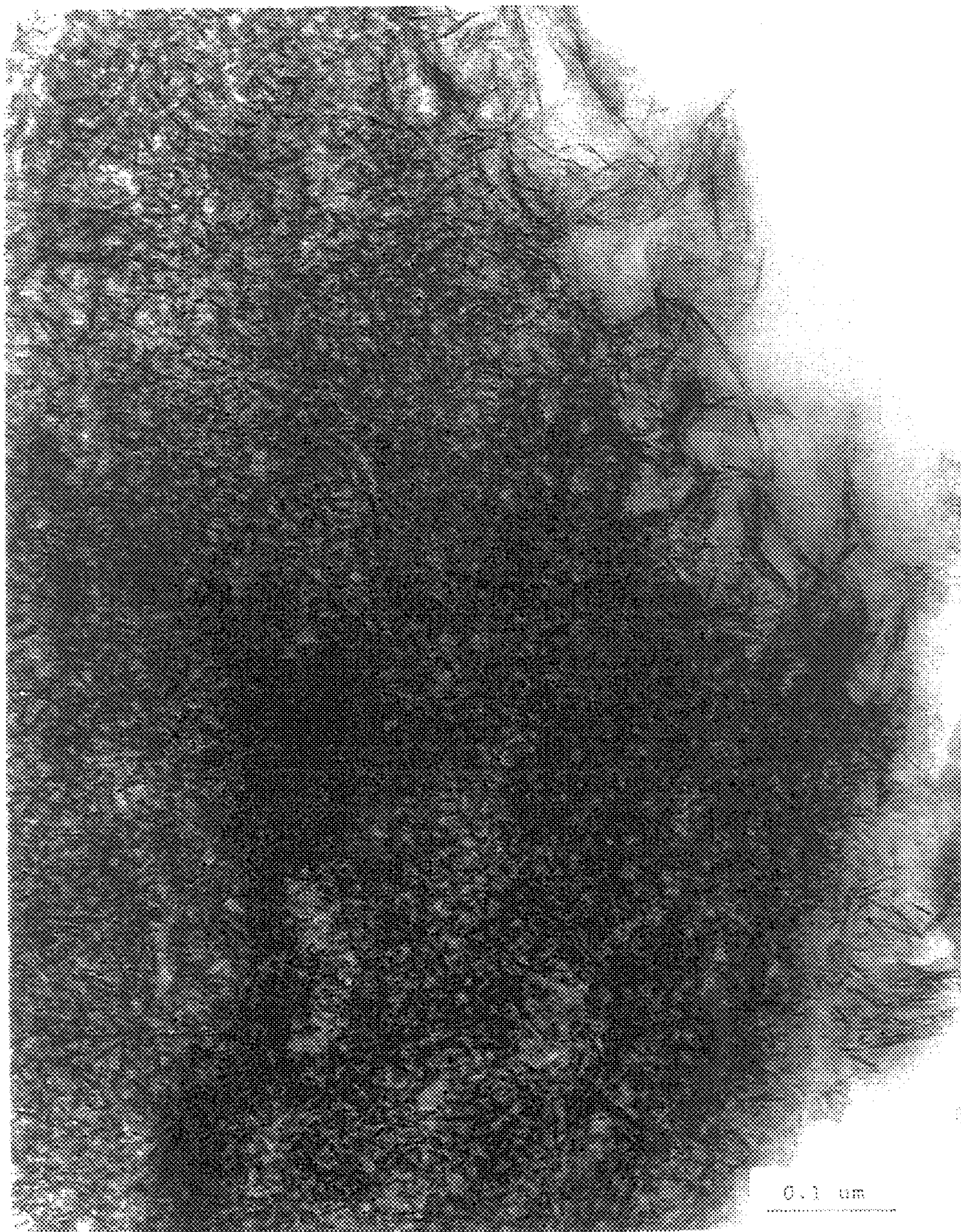
Figure 3 TEM picture of the 12%Zr/ \gamma -Al 2 O 3 sample after calcination in air at 600°C Support impregnated with ZrO(NO 2 ) 2 /citric acid
