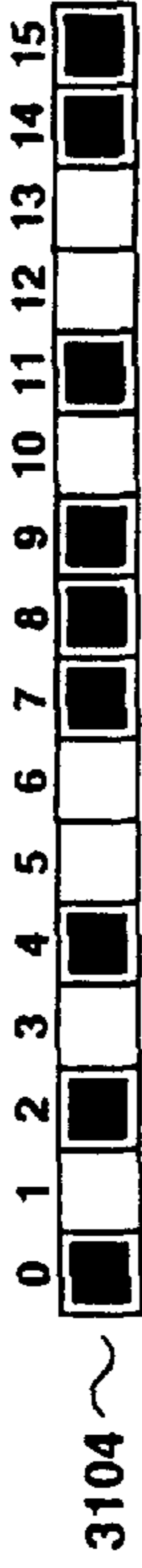
SCALED IMAGE ROW IN STANDARD BINARY BIT REPRESENTATION (WHITE RUNS)
