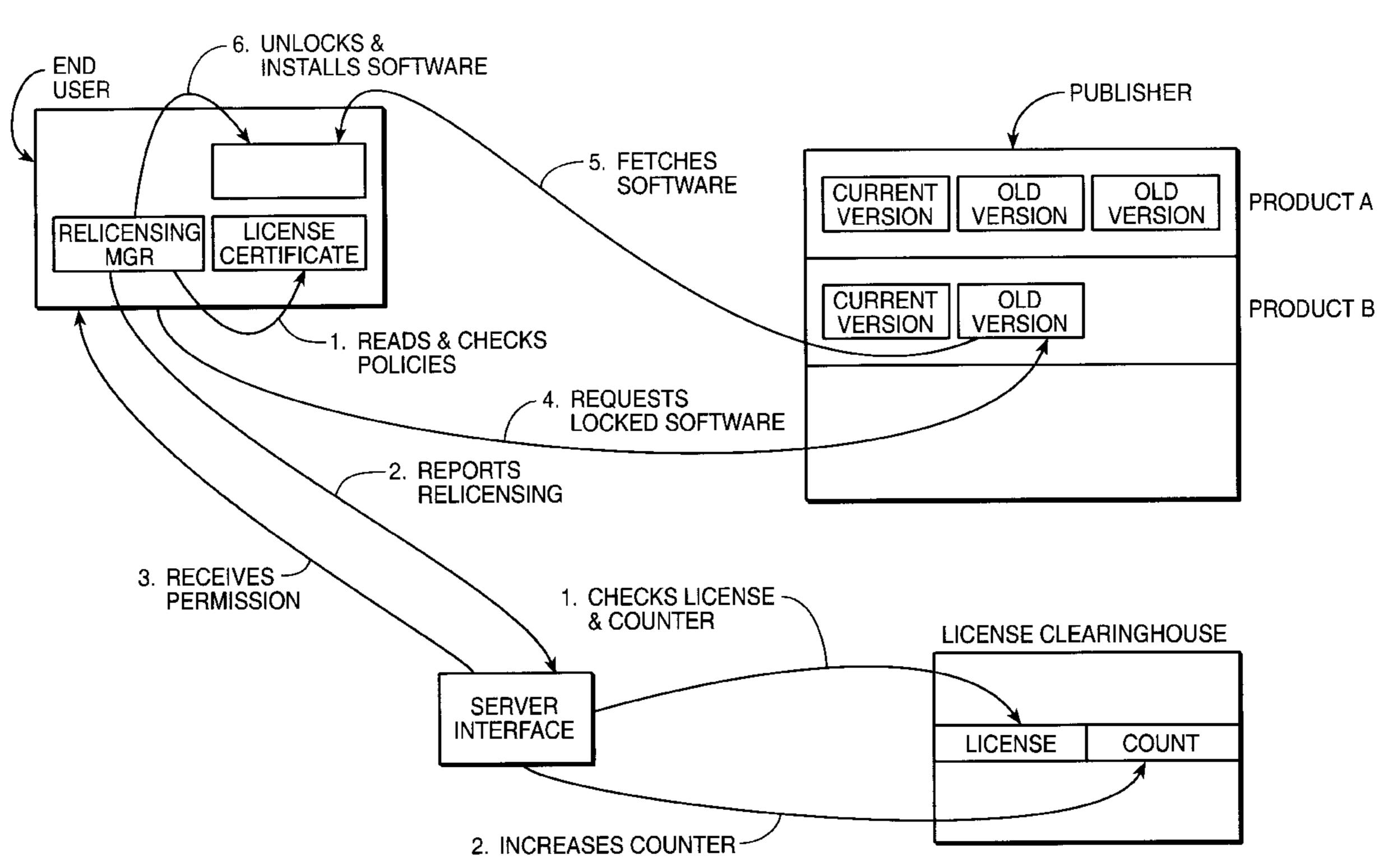
PRODUC CLEARINGHOUSE BLISHER OLD VERSION OLD VERSION LICENSE CURRENT VERSION REQUESTS LOCKED SOFTWARE 1. CHECKS LICENSE & COUNTER RELICENSING FETCHES SOFTWARE 2. INCREASES വ SERVER INTERFACE REPORTS RELICENSING 4. READS & CHECKS POLICIES UNLOCKS & INSTALLS SOFTWARE  $\dot{\alpha}$ LICENSE CERTIFICATE RECEIVES / PERMISSION 6 G က
