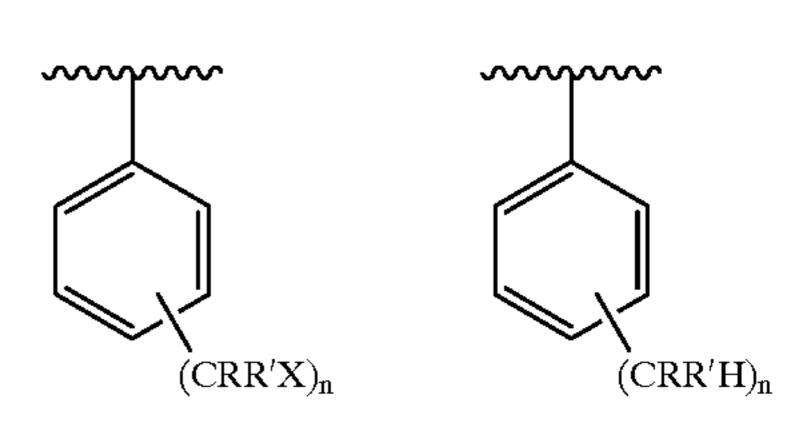
wherein R and R' are independently selected from the group consisting of hydrogen and C<sub>1</sub> to C<sub>4</sub> alkyl, a X is bromine or chlorine, n is 1–3 and wherein the halogen content of the copolymer is 7 mole % or less and the halogen content of the backbone polymer is 2 mole % or less;
