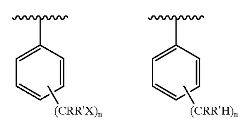
wherein R and R' are independently selected from the group consisting of hydrogen and  $C_1$  to  $C_4$  alkyl, a X is bromine or chlorine, n is 1–3 and wherein the halogen content of the copolymer is 7 mole % or less and the halogen content of the backbone polymer is 2 mole % or less.
