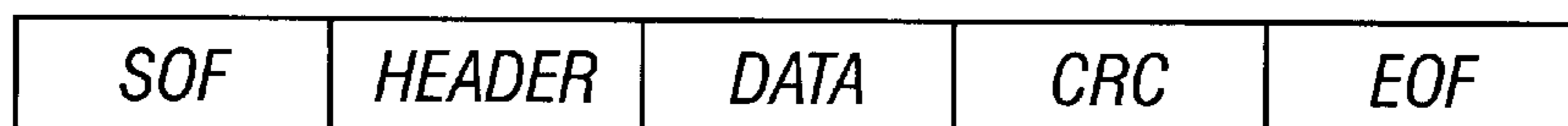
FIBRE CHANNEL FRAME
