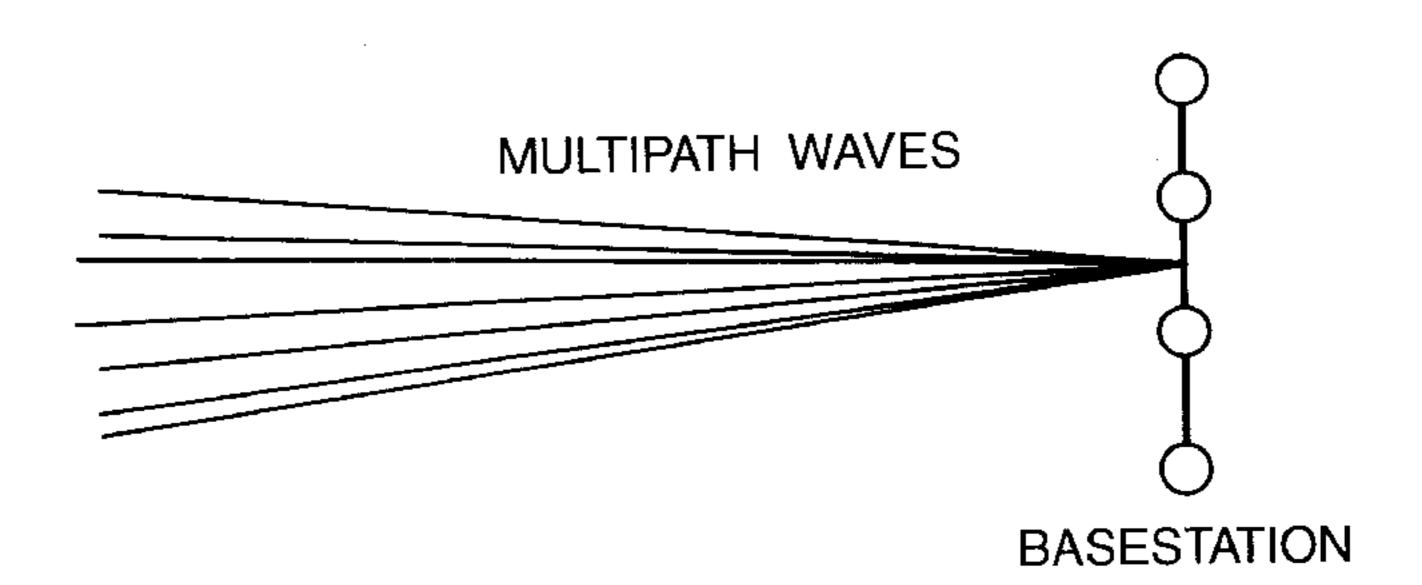
A SIGNAL TRANSMITTED FROM THE MOBILE REACHES THE BASESTATION HAVING TRAVELLED VIA A NUMBER OF PATHS WHICH EXIST AS A RESULT OF SCATTERING FROM OBSTACLES RANDOMLY DISTRIBUTED ON A CIRCLE SURROUNDING THE MOBILE
