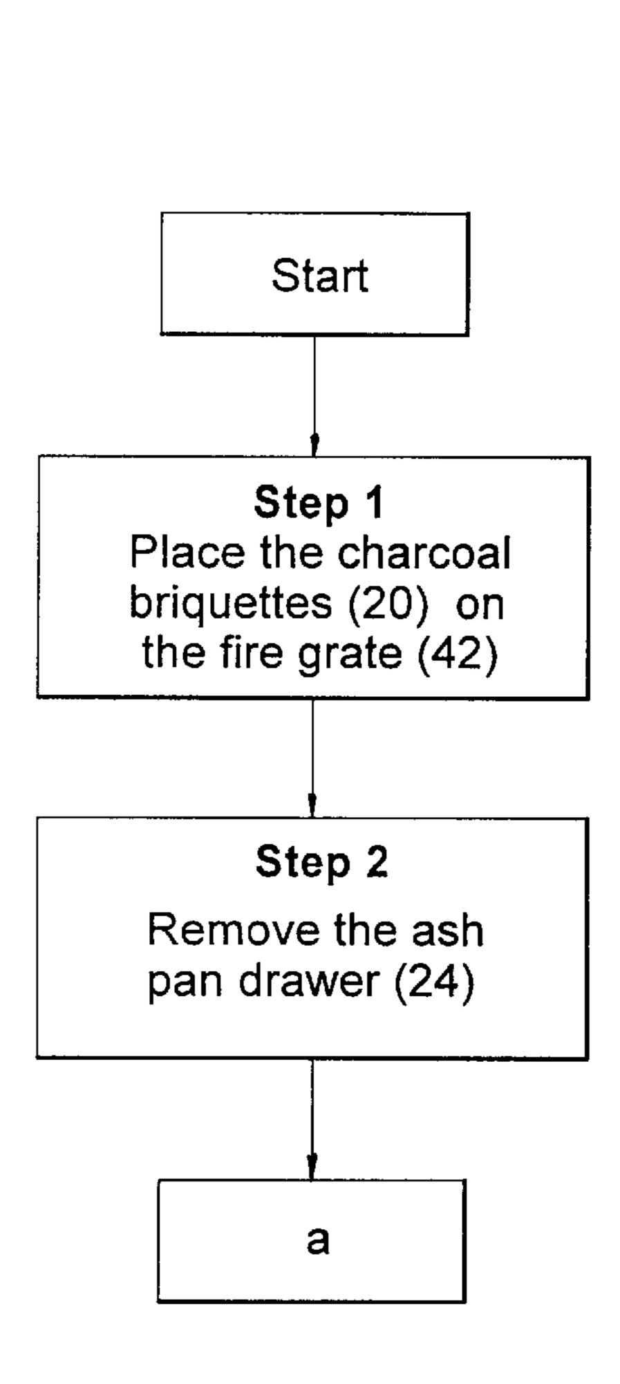
Method of utilizing the combination gas and charcoal grill (10, 110, 210) for cooking food using the charcoal briquettes (20) as a heat source.
