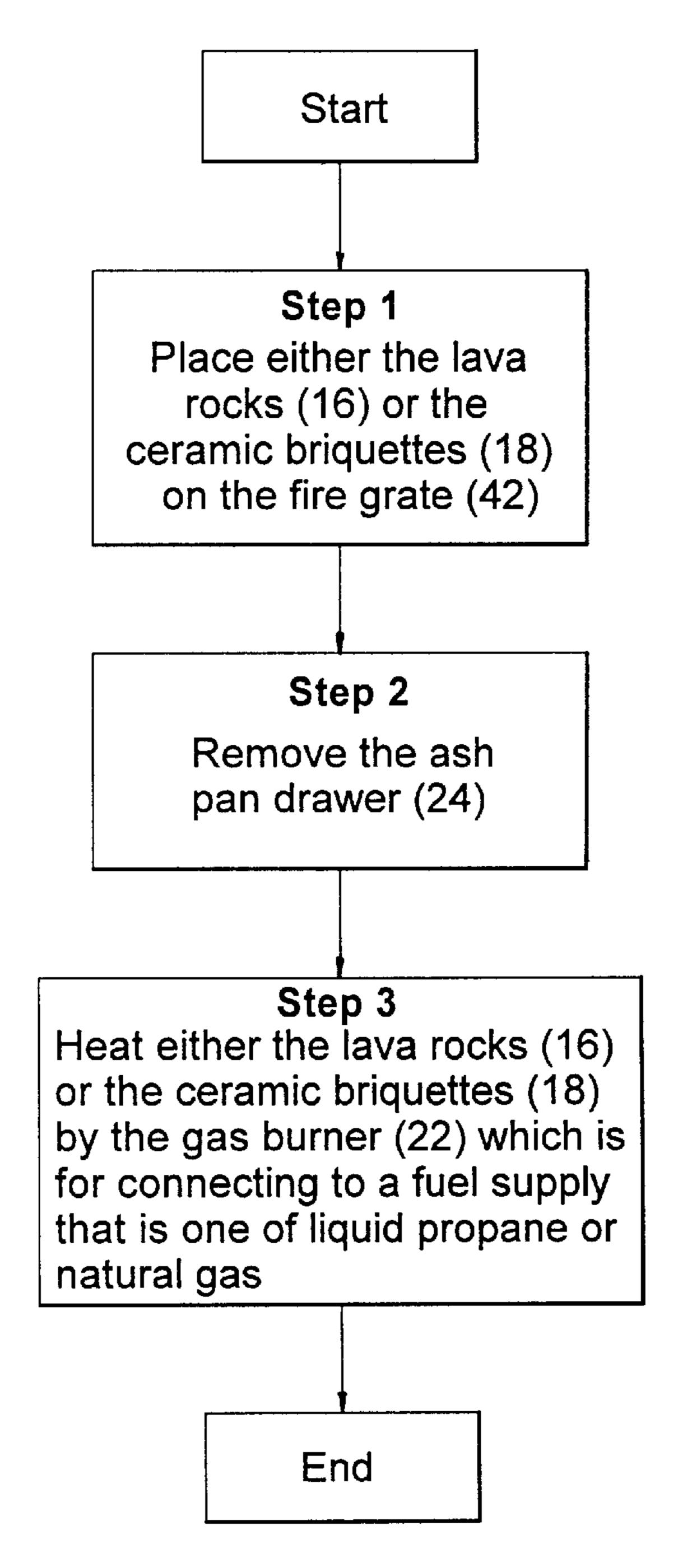
Method of utilizing the combination gas and charcoal grill (10, 110, 210) for cooking food using either the lava rocks (16) or the ceramic briquettes (18) as a heat source
