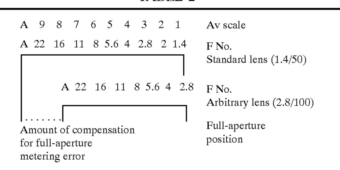
Table 2 indicates a case where a lens with an F No. of 2.8 and focal length of 100 mm is mounted, for example, as an 25 arbitrary other lens shown in Table 1. For example, when the full-aperture F No. of the arbitrary lens is selected to be "8", the calculation described above is executed upon deeming that the full-aperture F No. 4 was selected with the standard lens.
