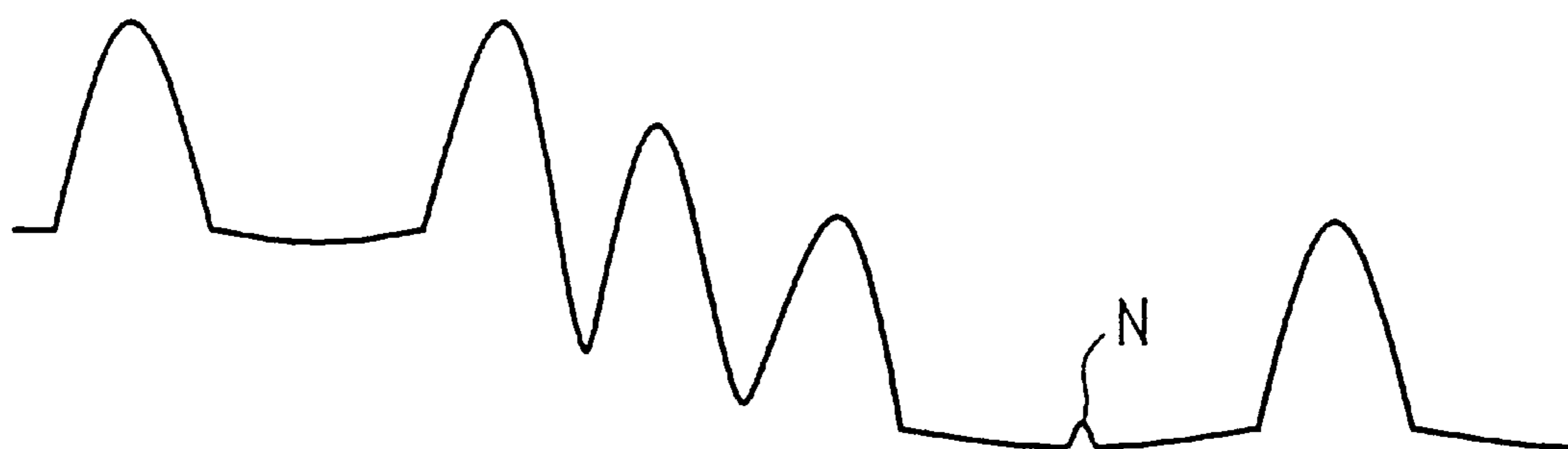
FIG. 3A Cutoff frequency low (large time constant)
