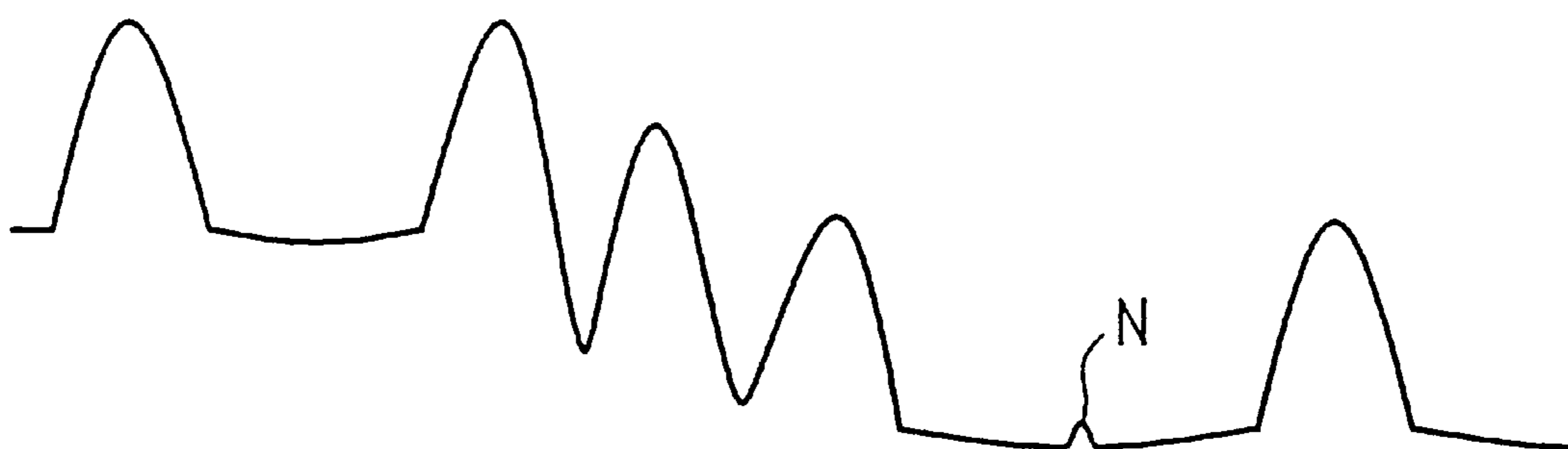
FIG. 3A Cutoff frequency low (large time constant)
