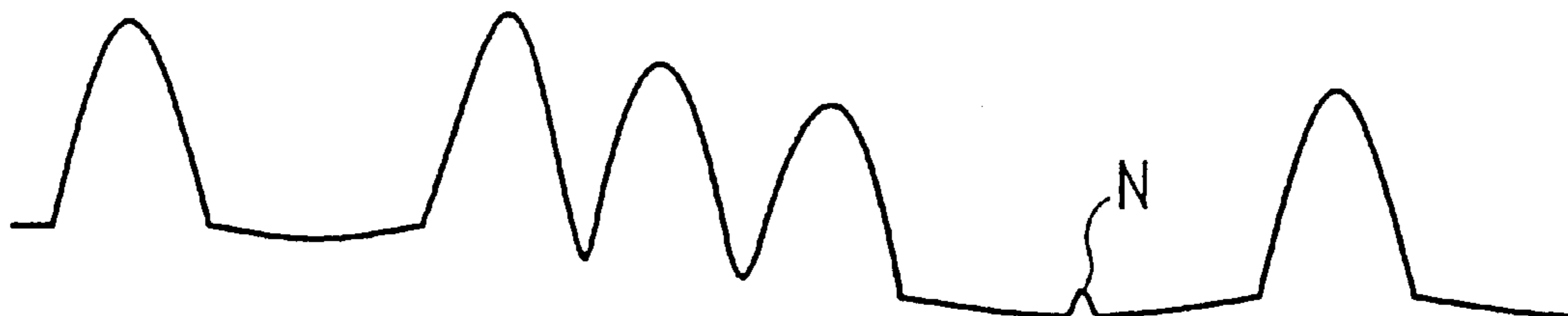
FIG. 3B Cutoff frequency high (small time constant)
