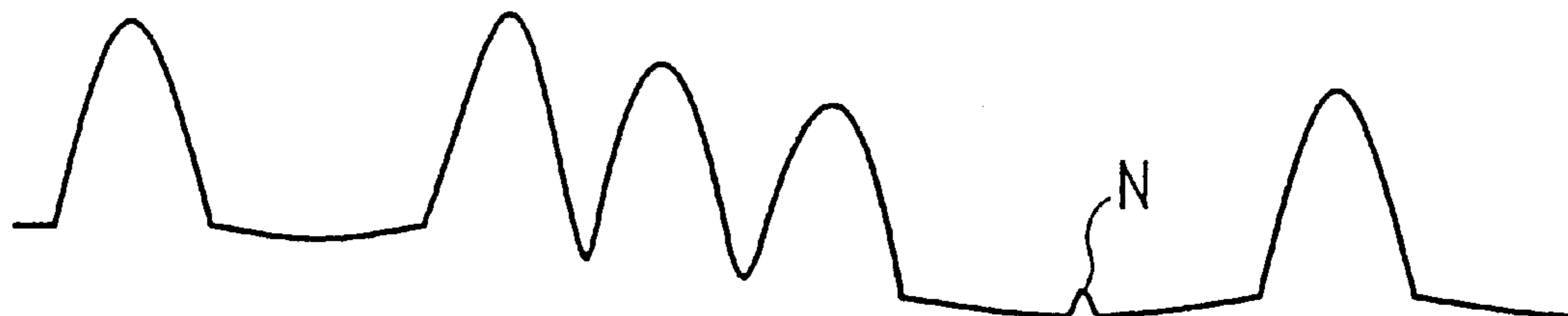
FIG. 3B Cutoff frequency high (small time constant)
