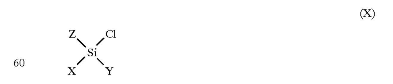
(wherein, X Y and Z denote independently tertiary butyl radicals or aryl radicals), and thereafter furthermore with zinc chloride or a zinc chloride complex.
