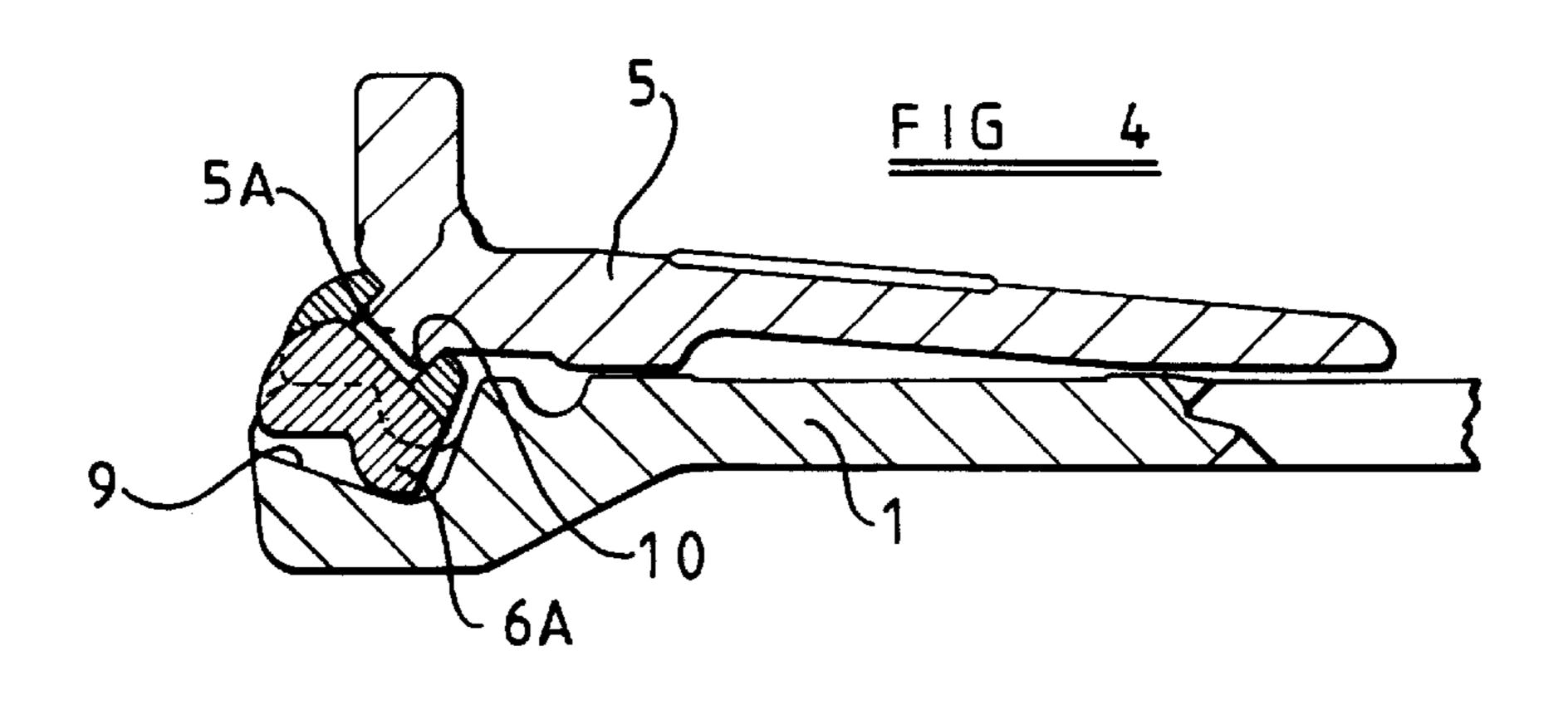
This invention relates to a vehicle wheel rim, primarily for heavy off-highway vehicles such as earth movers and of the general kind having a rim base carrying a pair of bead 5 retaining flanges, one of which is on or incorporated in a separate bead seat ring releasably retained, in use, on the rim base by a locking ring engaging a formation provided on the
